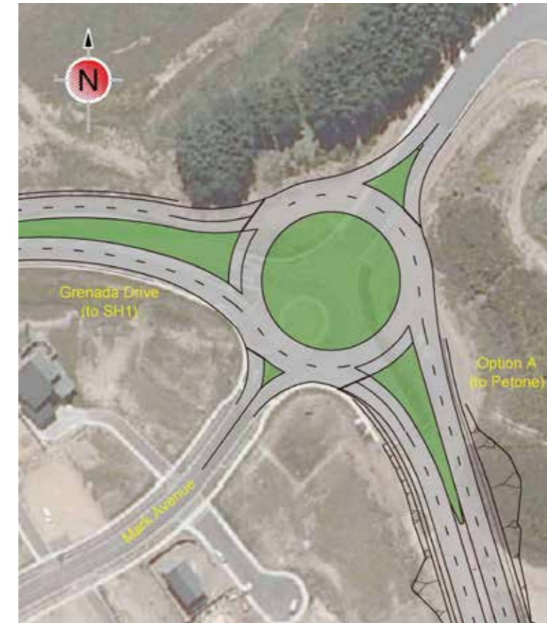
Figure 14-3: New Roundabout at Mark Avenue
