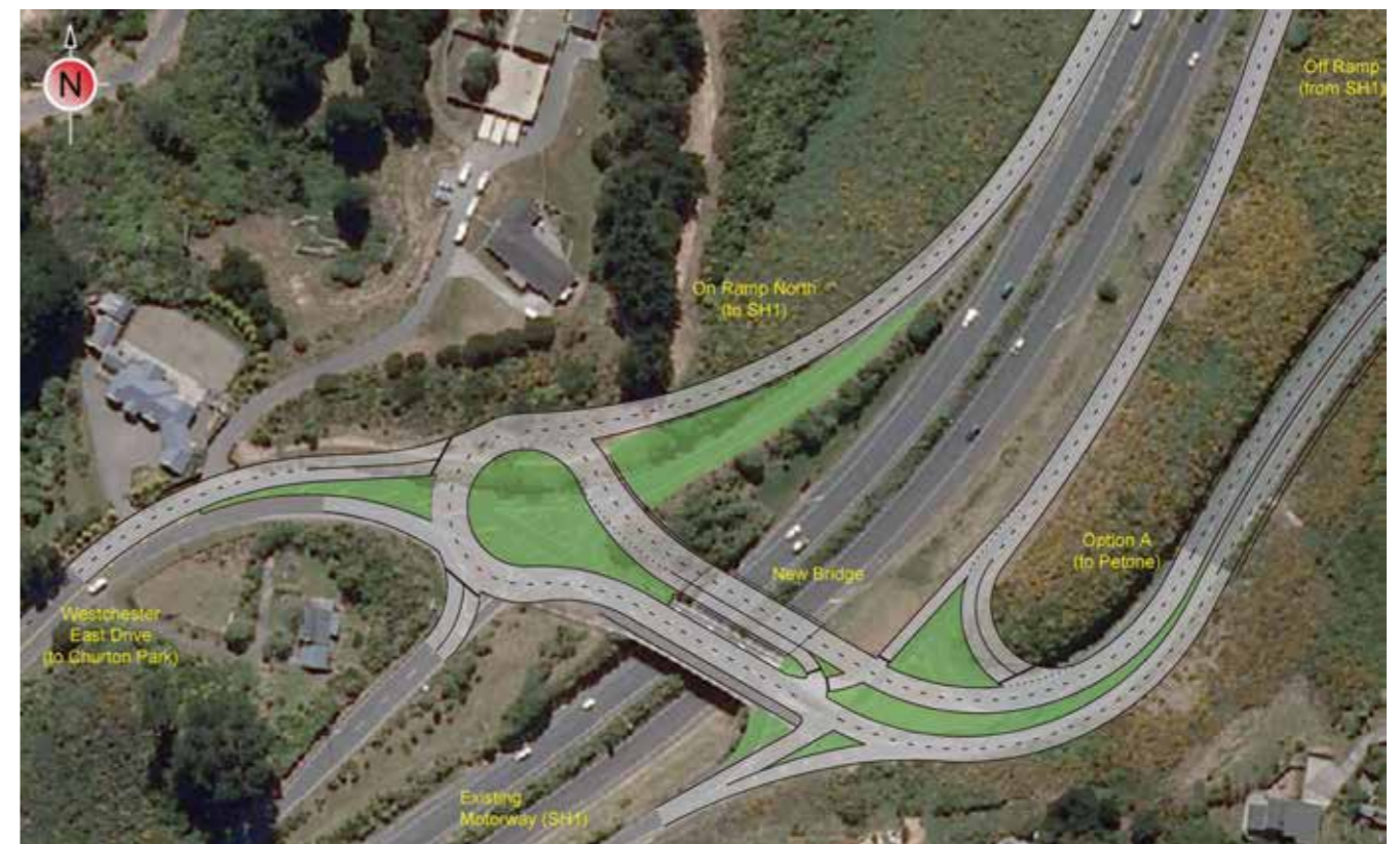
Figure 14-4: Upgraded Grenada Interchange at SH1
