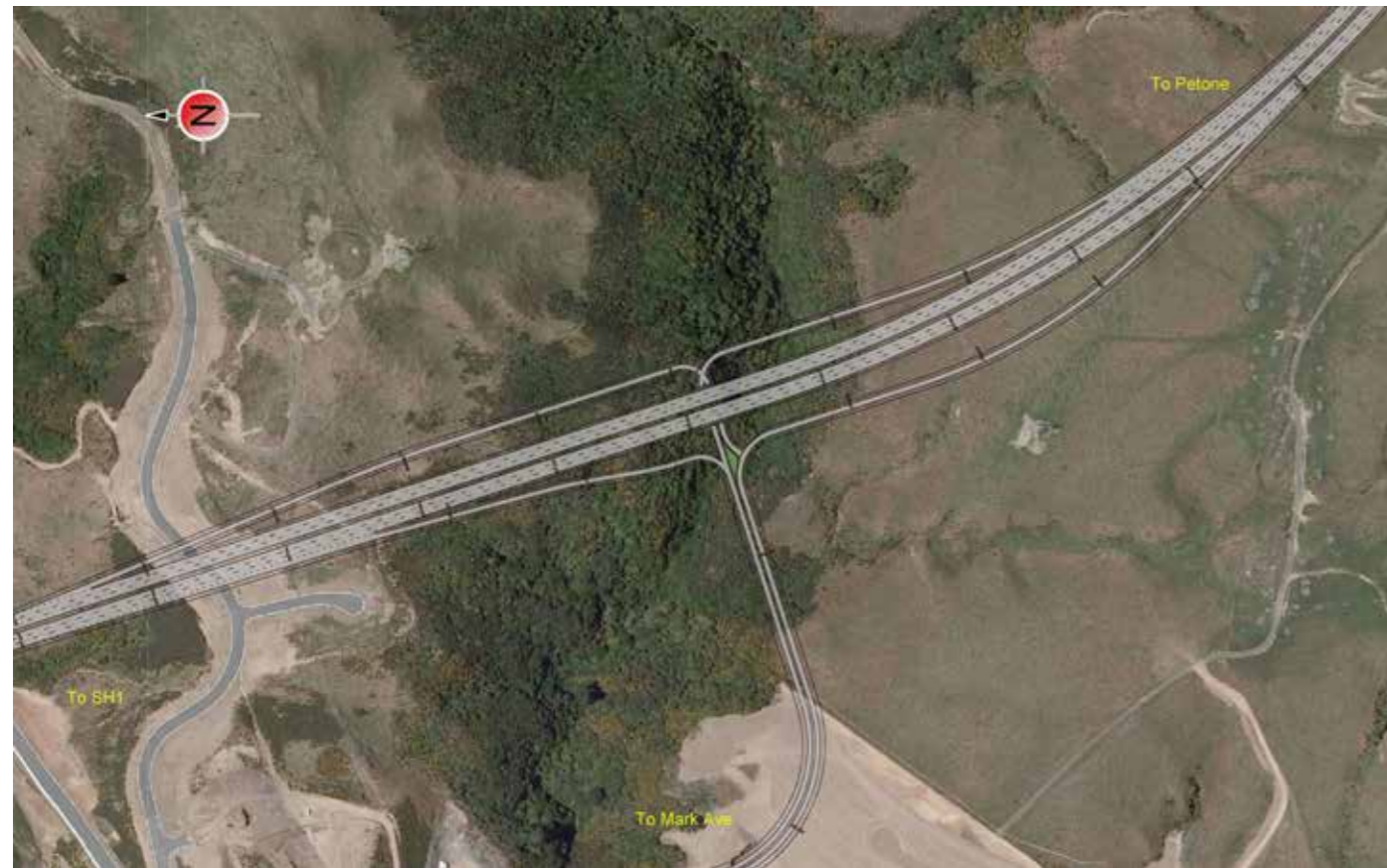
Figure 16-5: New Grade Separated Interchange to Mark Avenue
