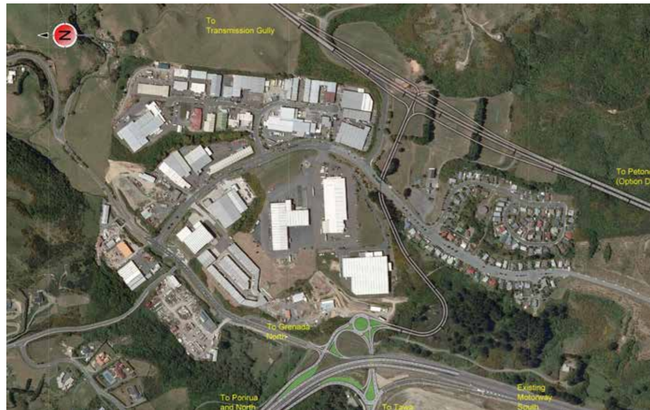
Figure 17-5: New Grade Separated Interchange to Tawa
