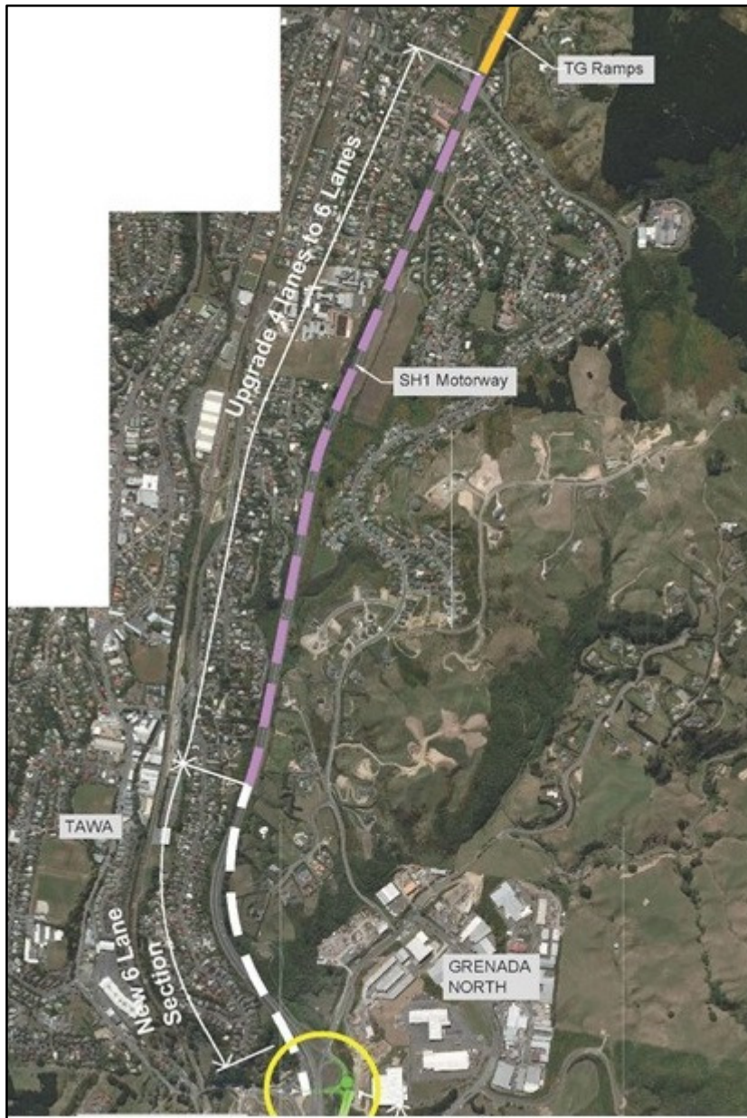
Figure 2k – Option 7 (C) (Section 3) – 6 Laning SH1 with Full Shoulders and Extg Median
