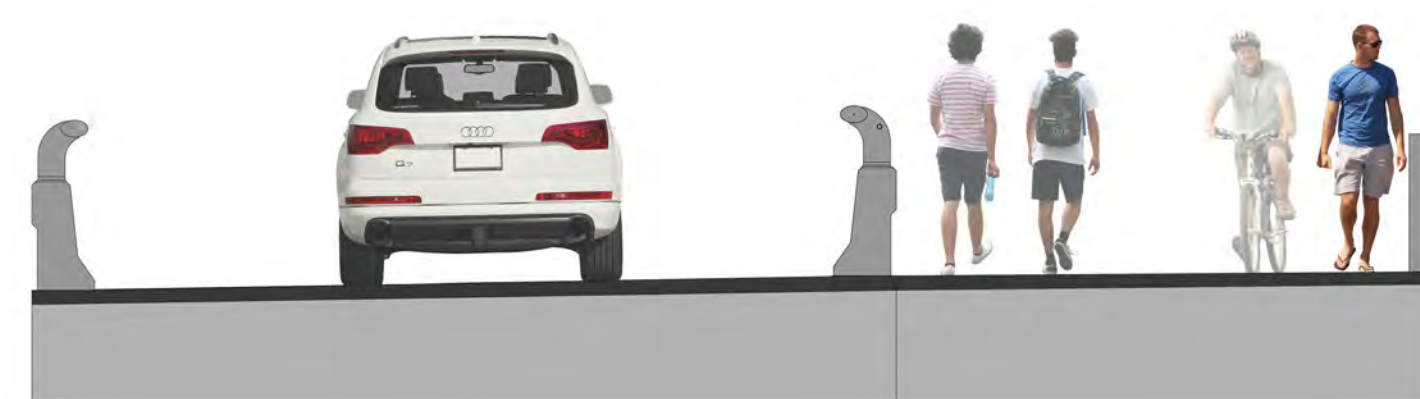
Artist's impression of single lane bridge with attached walking and wheeling path
