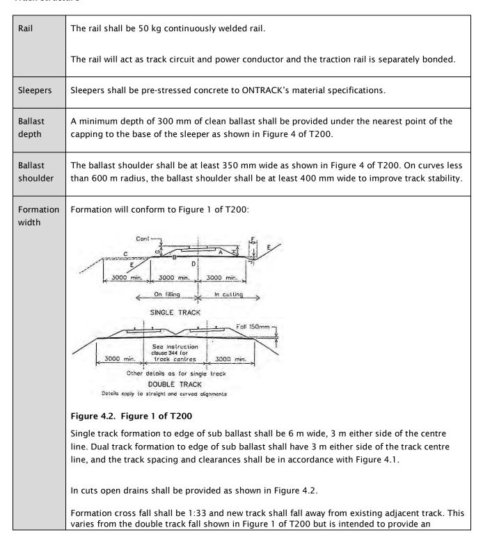
adequate cross slope whilst minimising the amount of ballast required and has been used in previous projects following agreement with KiwiRail.
