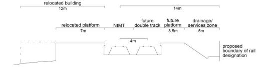
Figure 3.5. Provision for Otaki Station and future double tracking
