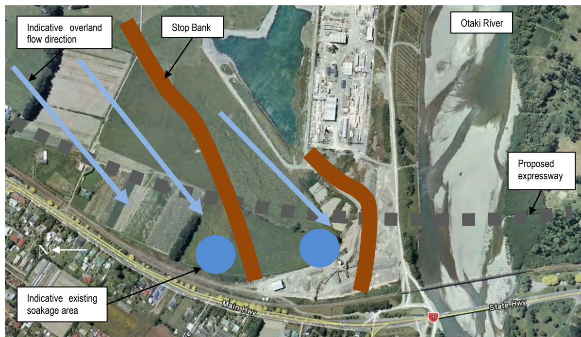
Figure 8 - location of existing soakage areas
