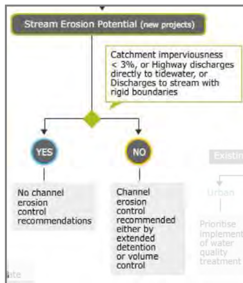
Figure 3 – Channel erosion control requirement selection process chart
