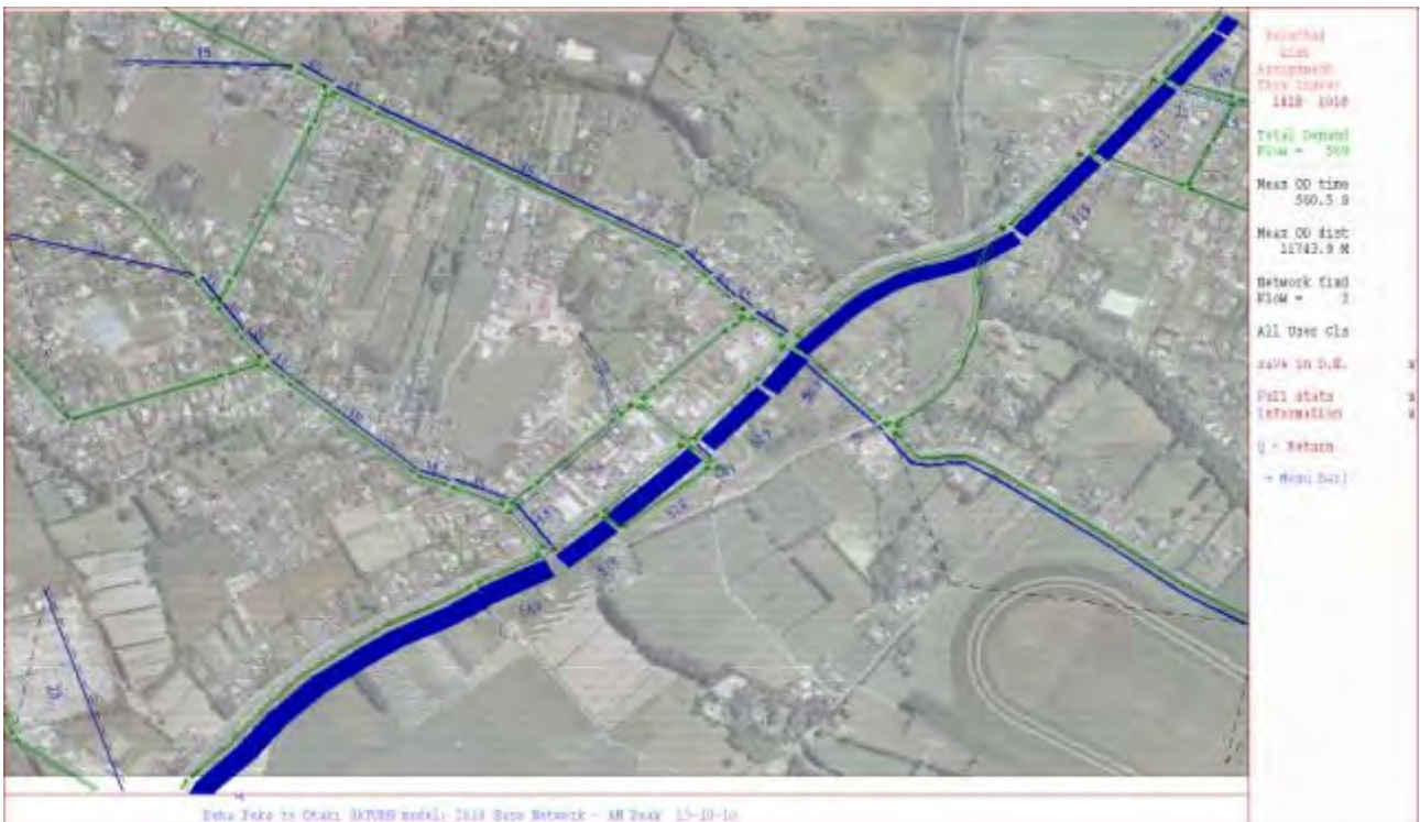
Otaki2010_SATURN Model_AM peak_Select Link_SH1 South of Waerenga Rd (SB)2
