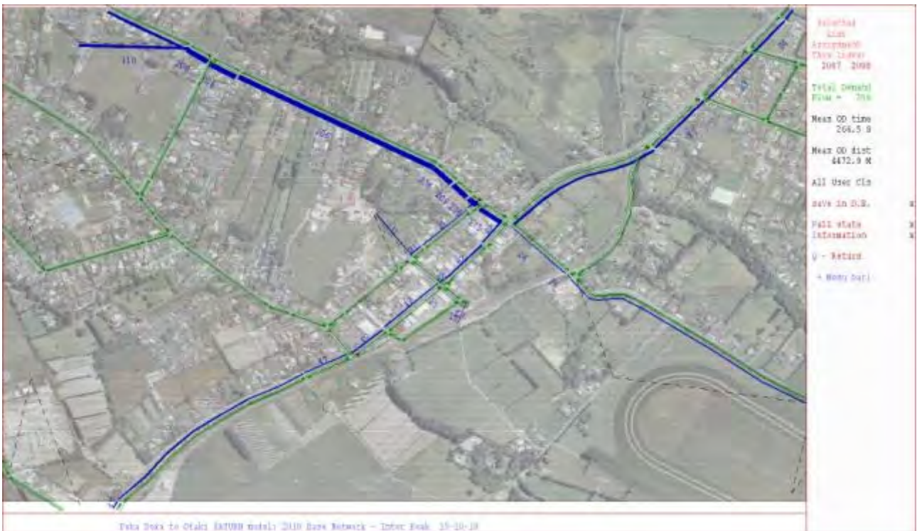
Otaki2010_SATURN Model_Inter peak_Select Link_Mill Rd West of Dunstan Rd (WB)2
