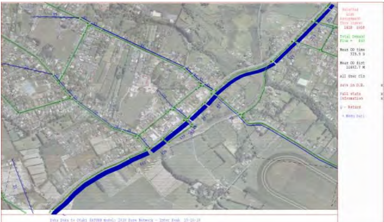
Otaki2010_SATURN Model_Inter peak_Select Link_SH1 South of Waerenga Rd (SB)2
