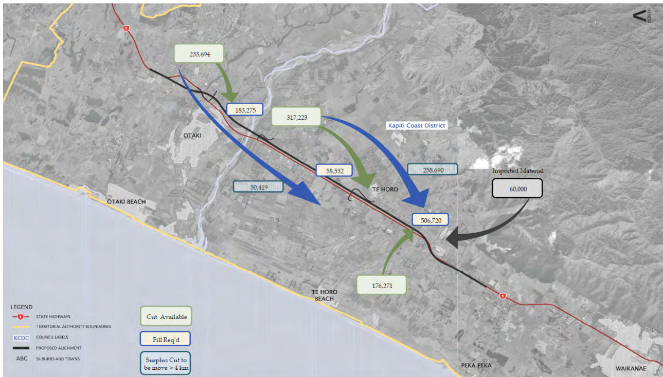
Figure 4-3: Earthworks Material Movement along Site
