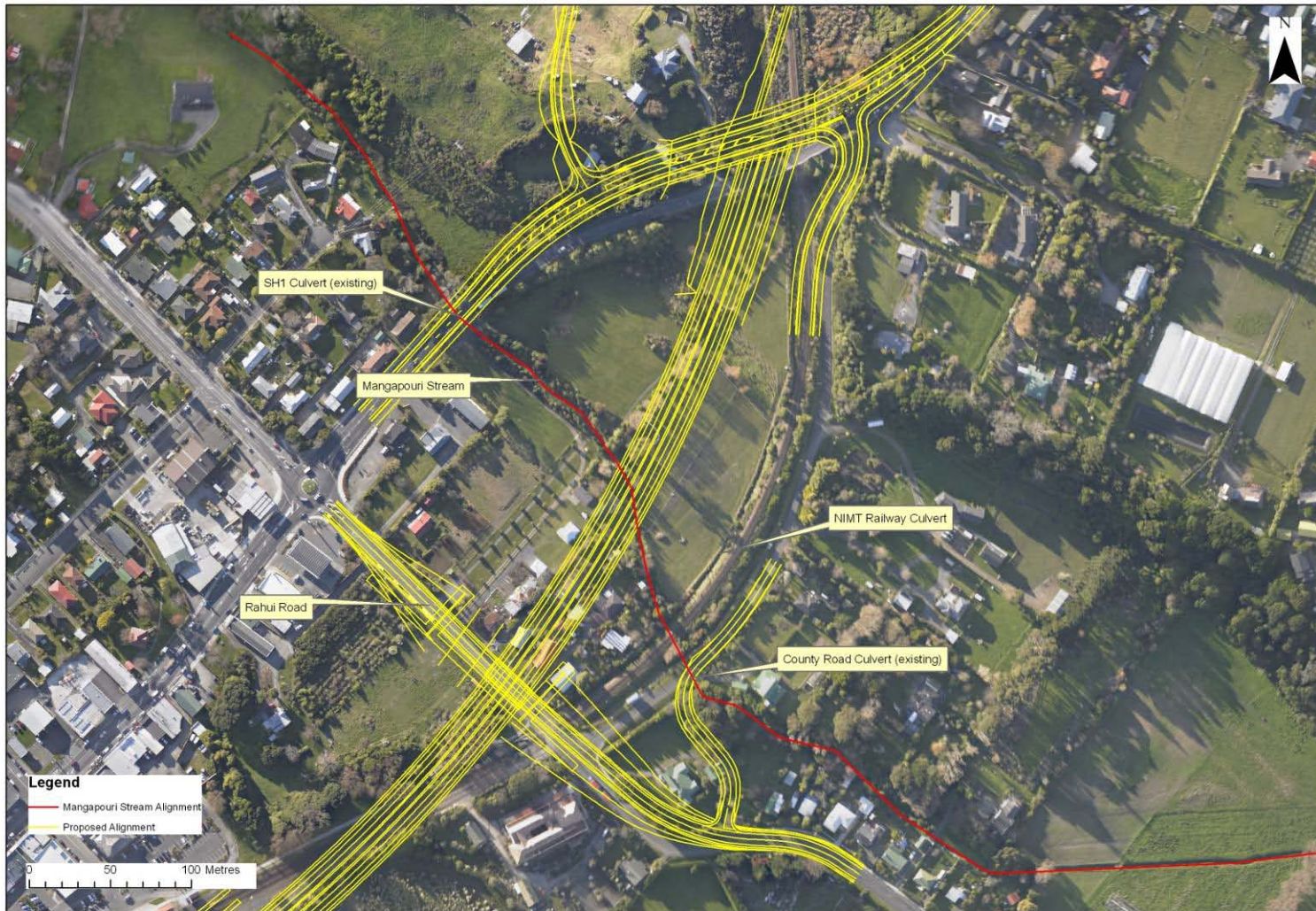
Figure 3 Existing culvert system along Mangapouri Stream in SH1 / County Rd / Rahui Rd triangle with footprint of proposed PP20 Expressway and relocated NIMT railway overlaid
