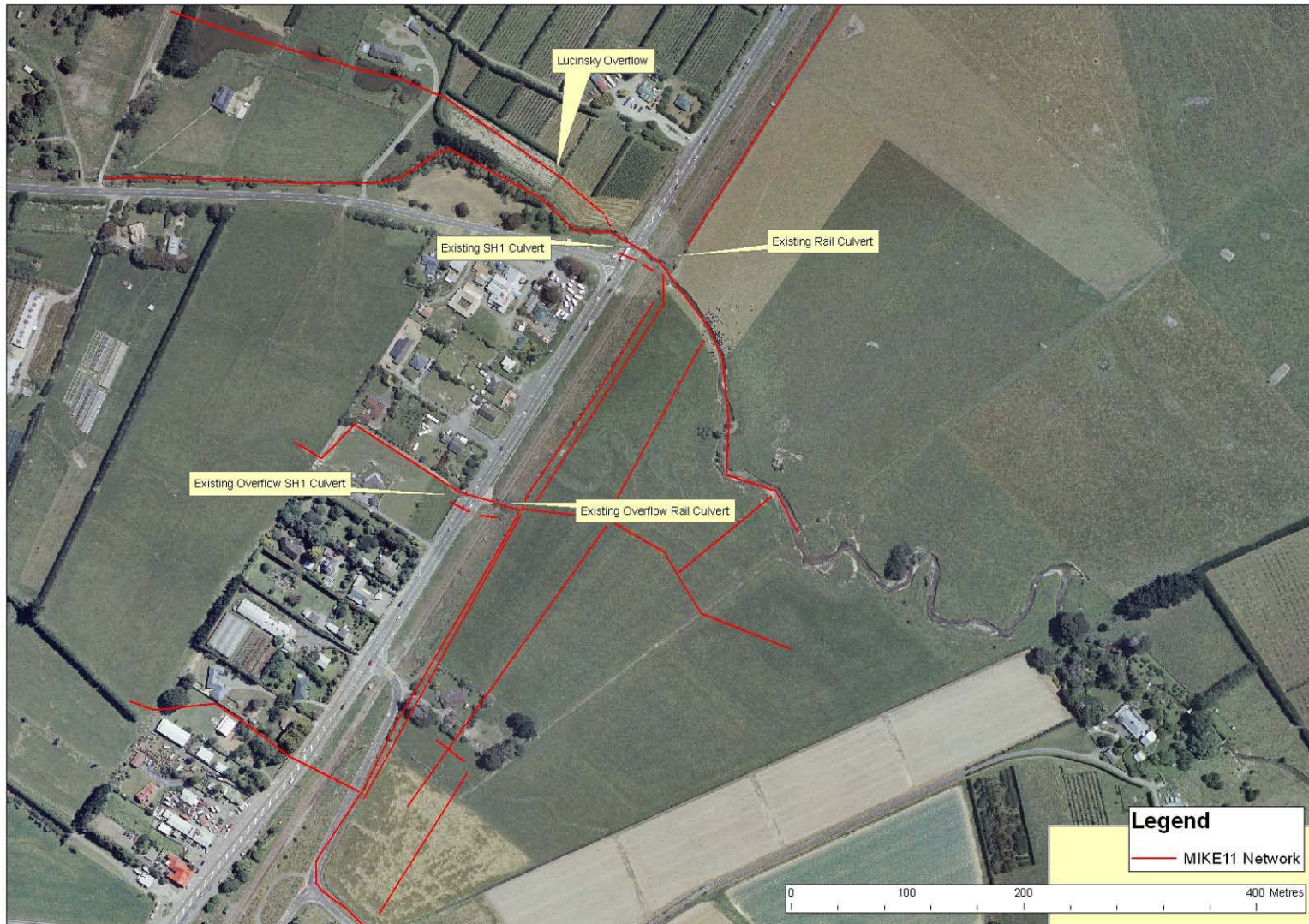
Figure 11 Existing SH1 and NIMT railway crossings of Mangaone Stream with layout of stream channel and secondary overland flow paths
