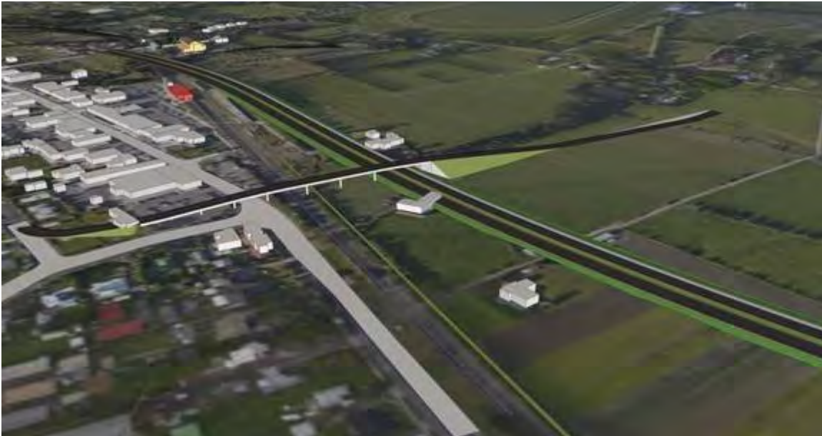
Figure 3.6 Perspective Illustration of Waerenga Rd Vehicular Bridge (Option EW4)
