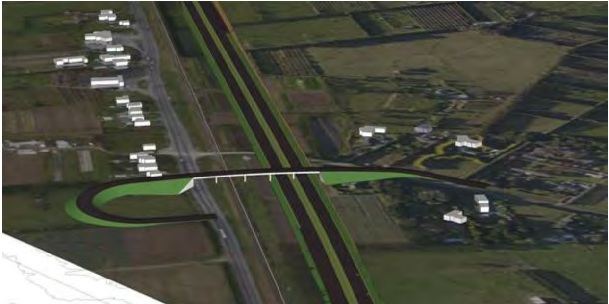
Figure 3.9 Perspective Illustration of Grade Separated Old Hautere Rd option (Option OH2)
