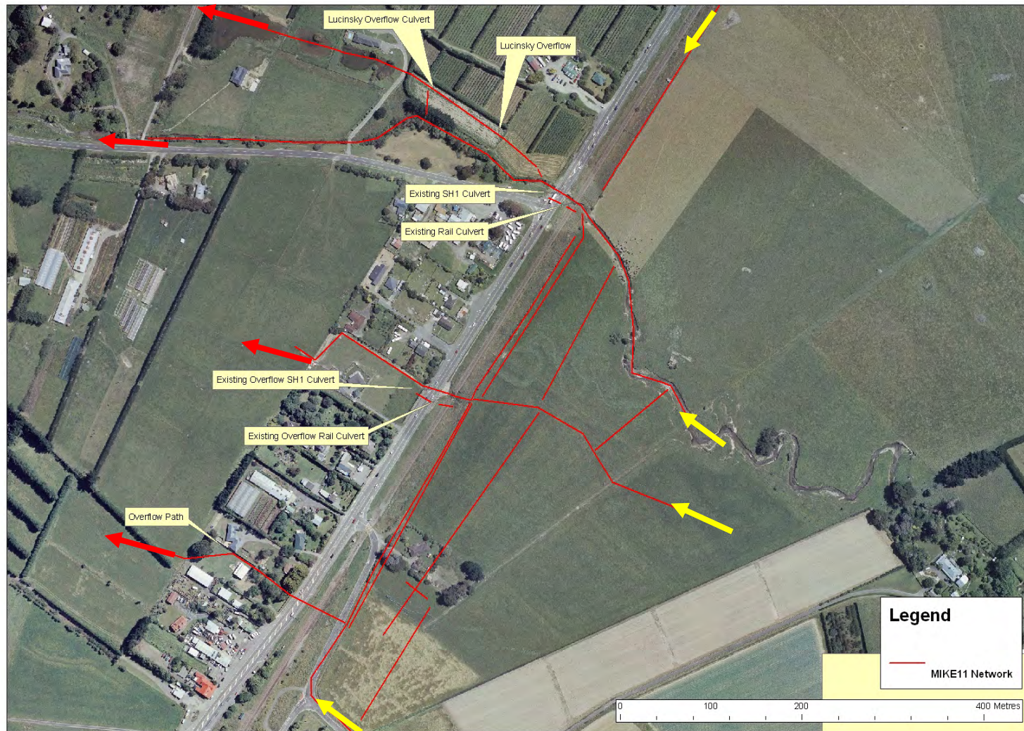
Figure 7.1 Existing SH1 and NIMT railway crossings of Mangaone Stream (layout of MIKE11 model network overlaid to indicate drainage paths (inflows indicated by yellow arrows, outflows by red arrows))
