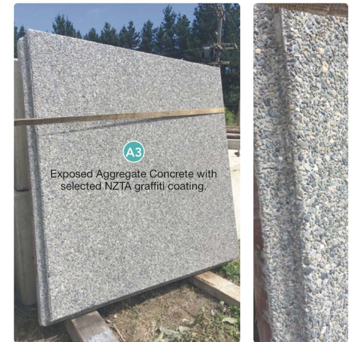
Figure 69. Image indicating size and proportion of RE panels at 2.0m x 2.0m.
