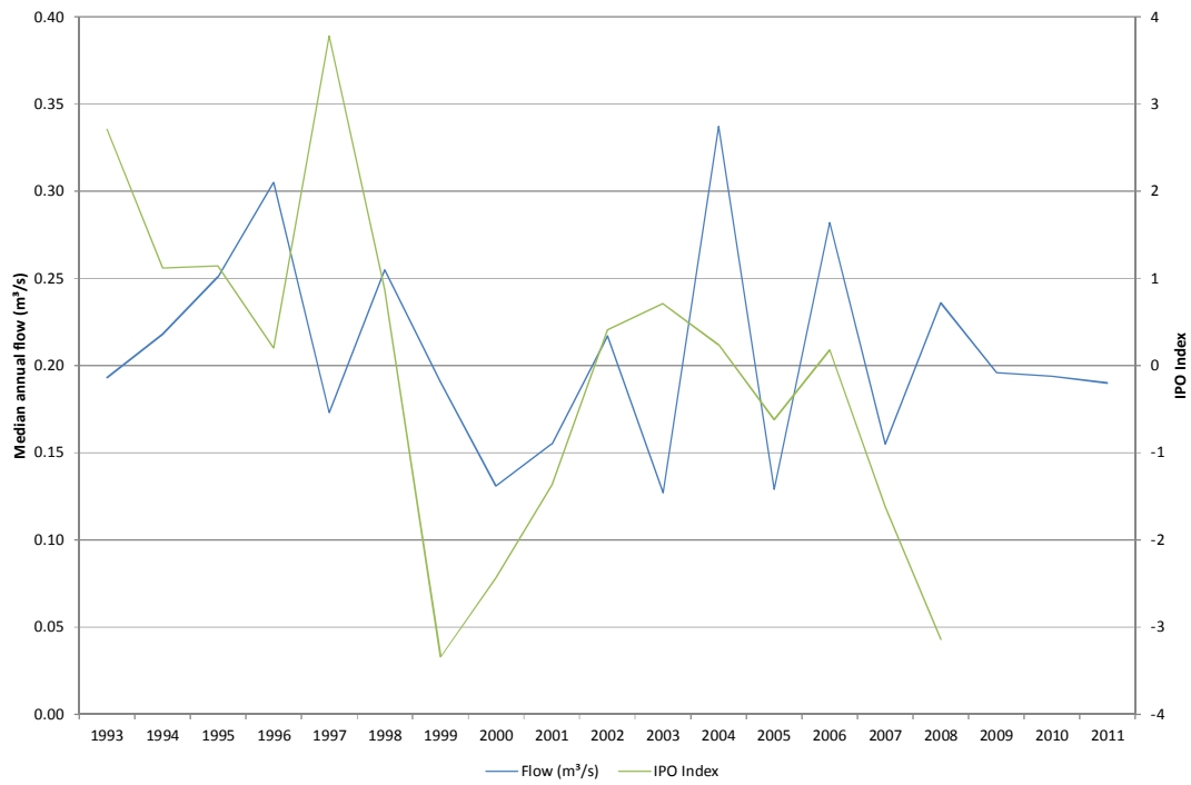
Figure 7: Comparison of the median annual flows in Mangaone Stream with variation in the IPO (1993-2012).
