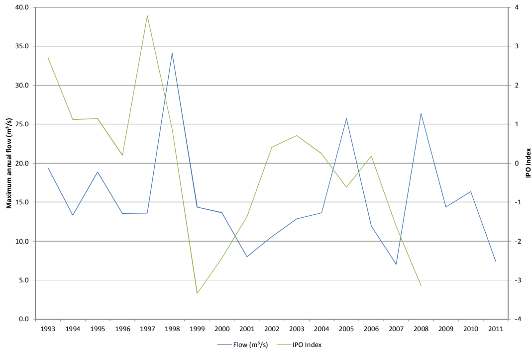
Figure 11: Comparison of the maximum annual flows in Mangaone Stream with variation in the IPO (1993-2012).
