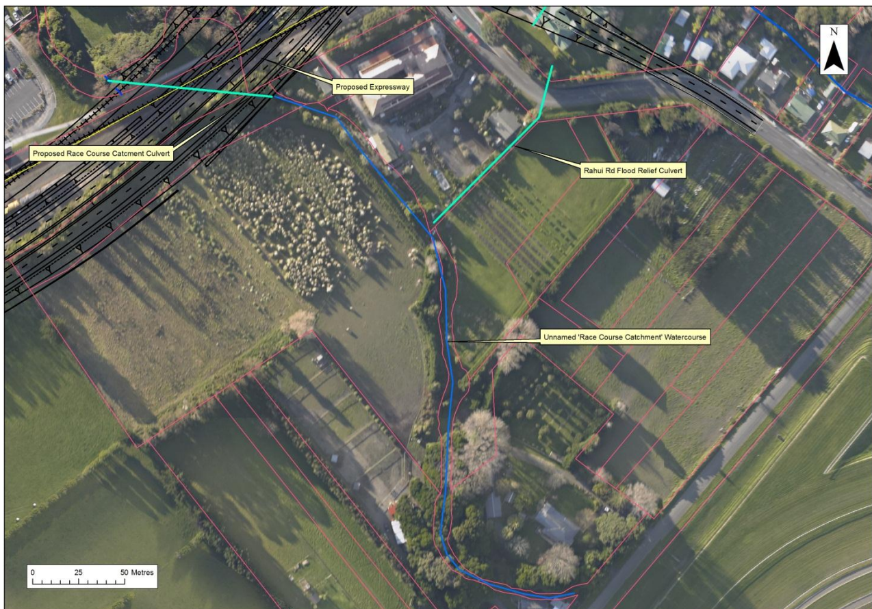
Figure 4-4 Aerial photograph showing drainage system for unnamed watercourse conveying storm runoff from part of Ōtaki Racecourse
