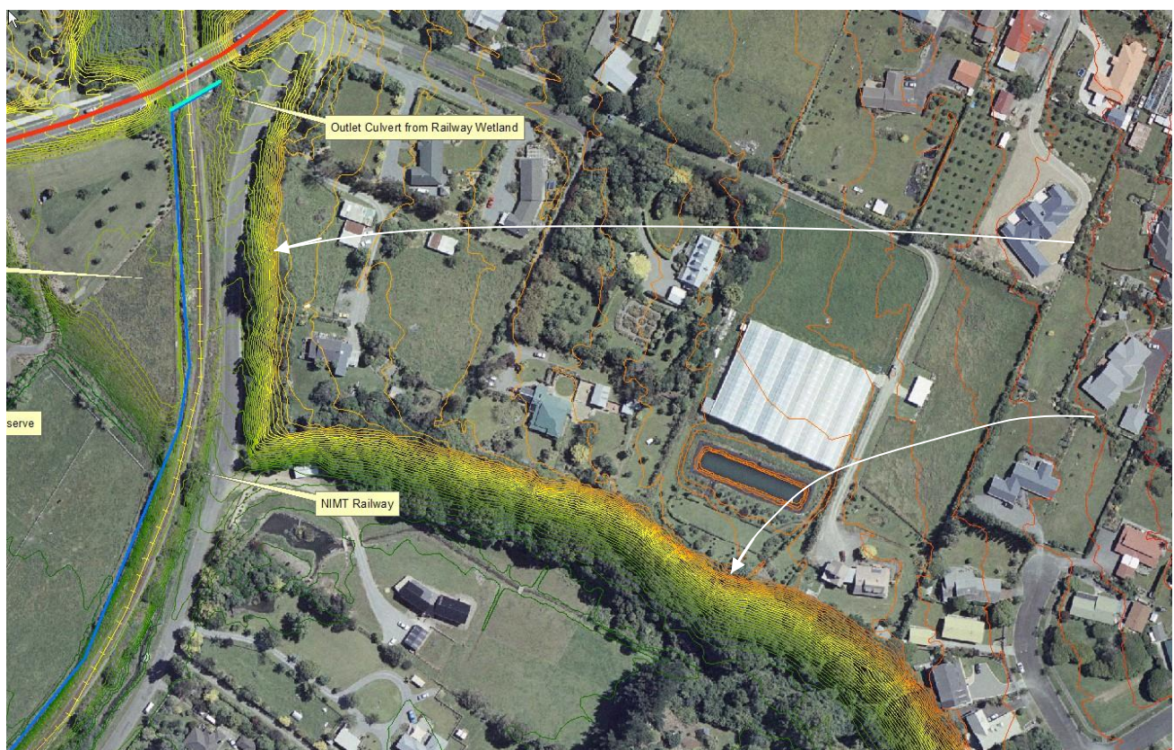
Figure 3-14 Ground level contours in lower part of Te Manuao Catchment (contours shown in orange and yellow). Arrows show general direction of overland flow from lower Te Manuao Catchment.
