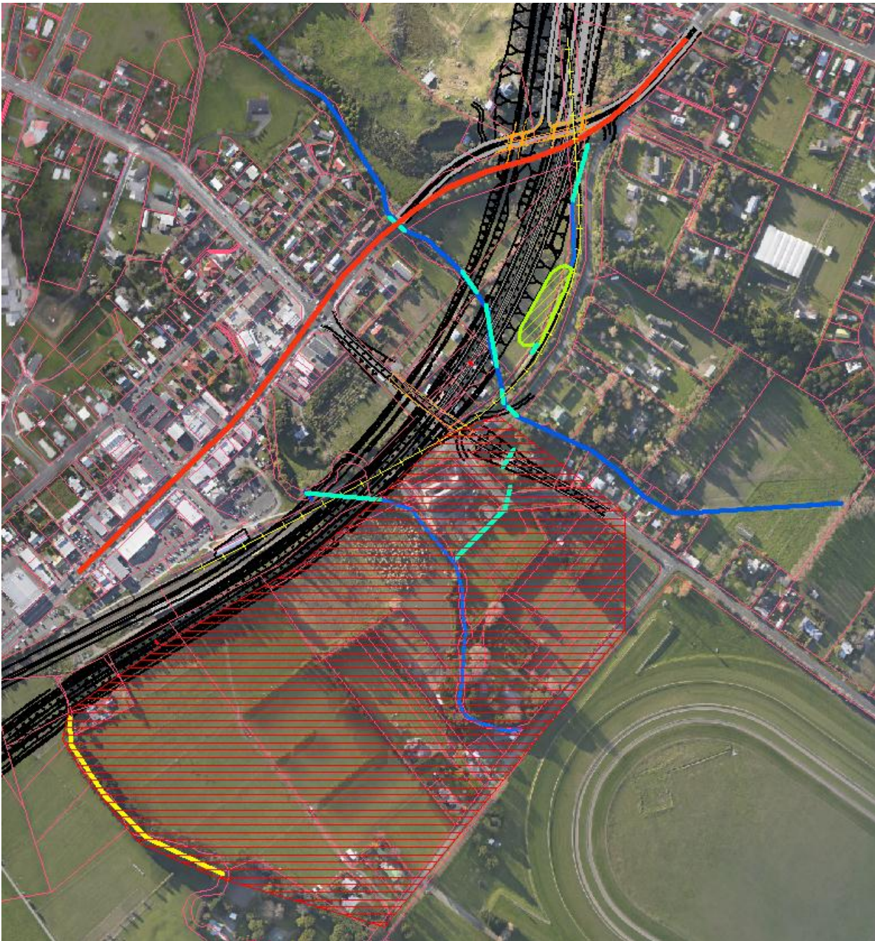
Figure F-2 Extent of MIKE21 model for proposed situation - model extent shown by red hatching, one-dimensional stream channel network in coupled MIKE11 model component indicated by blue lines, culverts indicated by aqua lines, secondary flood containment bund for Ōtaki River stopbank overflows indicated by yellow line
