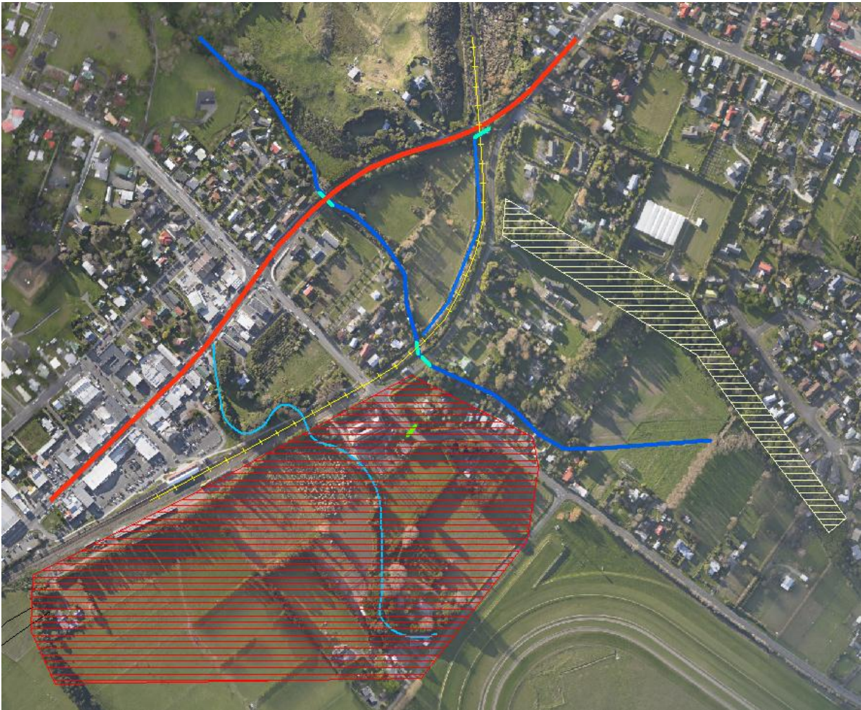
Figure F-1 Extent of MIKE21 model for existing situation – model extent shown by red hatching, one-dimensional stream channel network in MIKE11 model indicated by blue lines, culverts indicated by aqua lines
