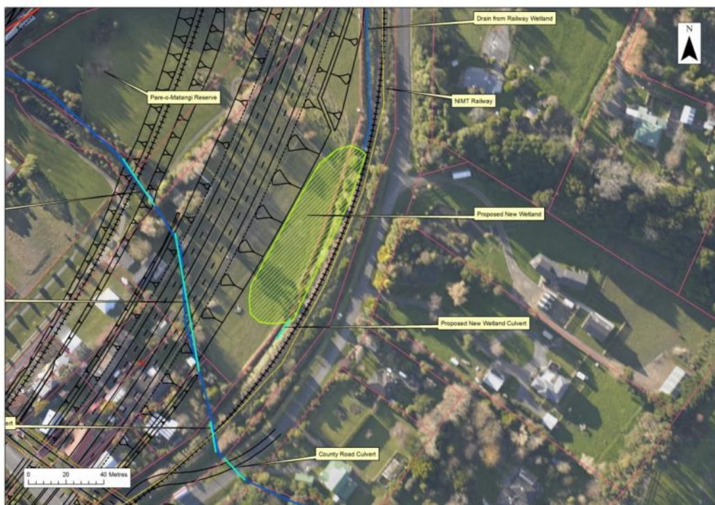
Figure 6-8 Aerial photograph of Railway Wetland area and drainage system with layout of proposed Expressway superimposed
