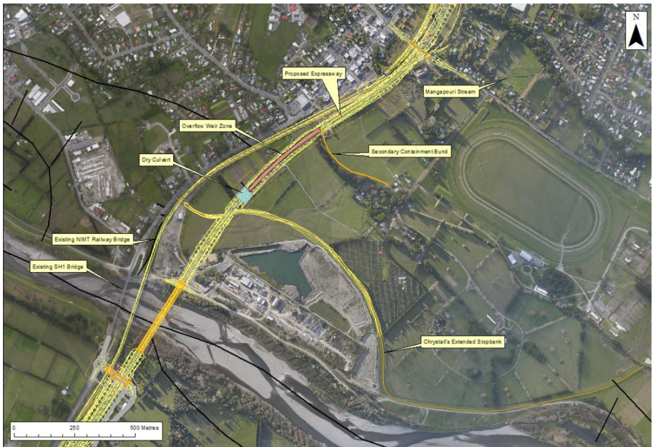
Figure 6-13 Proposed mitigation measures to reduce blocking effects of PP20 Expressway embankment on stopbank overtopping flows flowing across Ōtaki River floodplain
