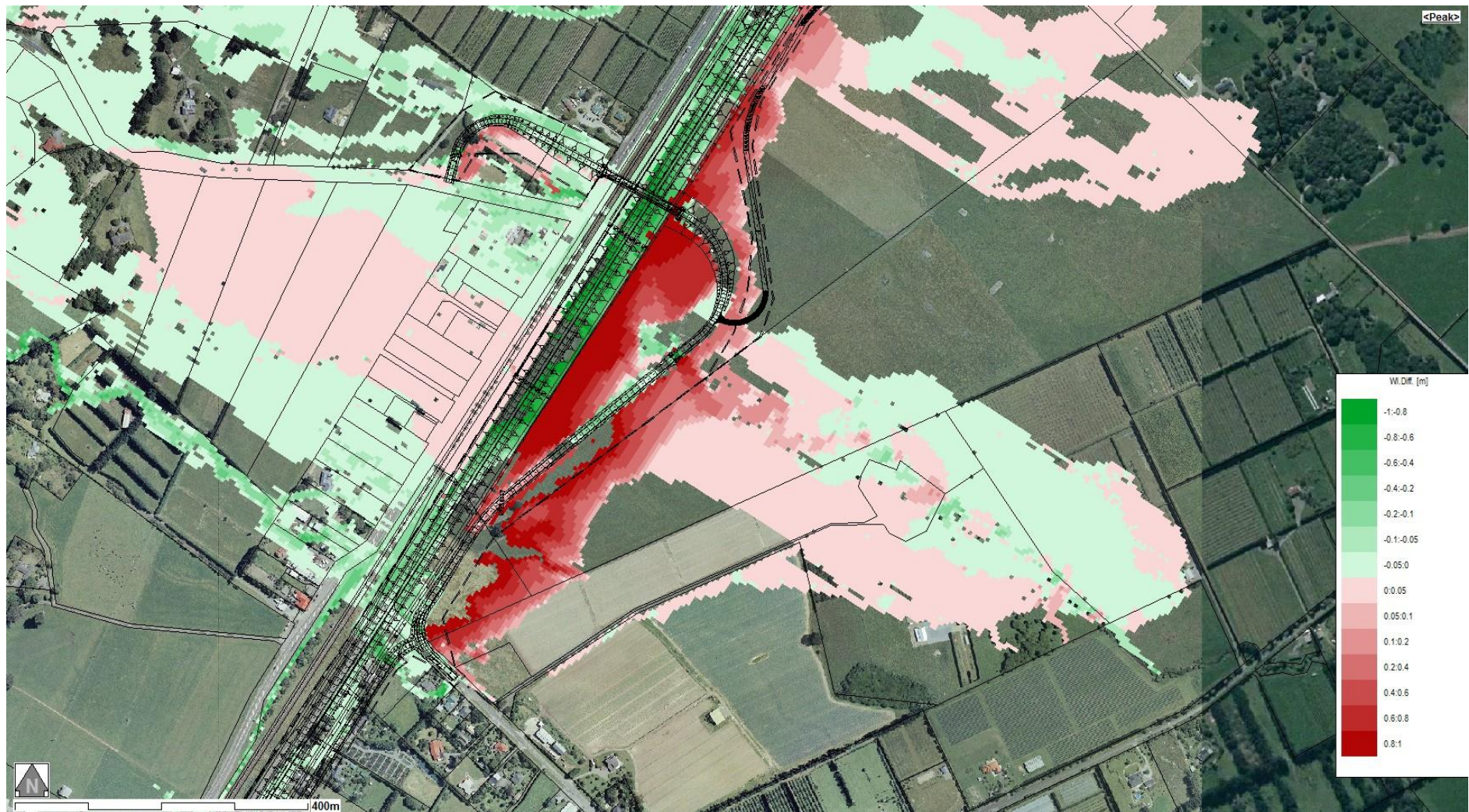
Figure 6-21 Changes in predicted peak flood depths across the Mangaone Stream alluvial fan and floodplain system between existing and proposed situations for 1% AEP flood adjusted for possible future climate change effects to 2090 (pink shading indicates areas of increased flow depths, green shading indicates areas of decreased flow depths)
