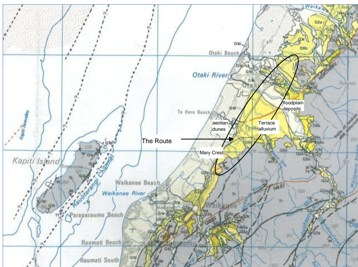
Illustration 3 - Geology of the area indicated on QMap (after IGNS, 2000a)
