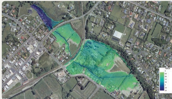
Flood map of existing situation for a 100-year return period (1-in-100 year)* flood upstream of State Highway 1 in the Mangapouri Stream.
