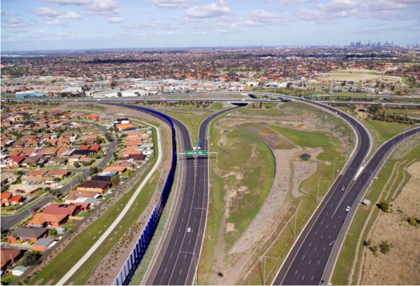
Figure 2 – System interchange (Source: AGRD Part 4C)
