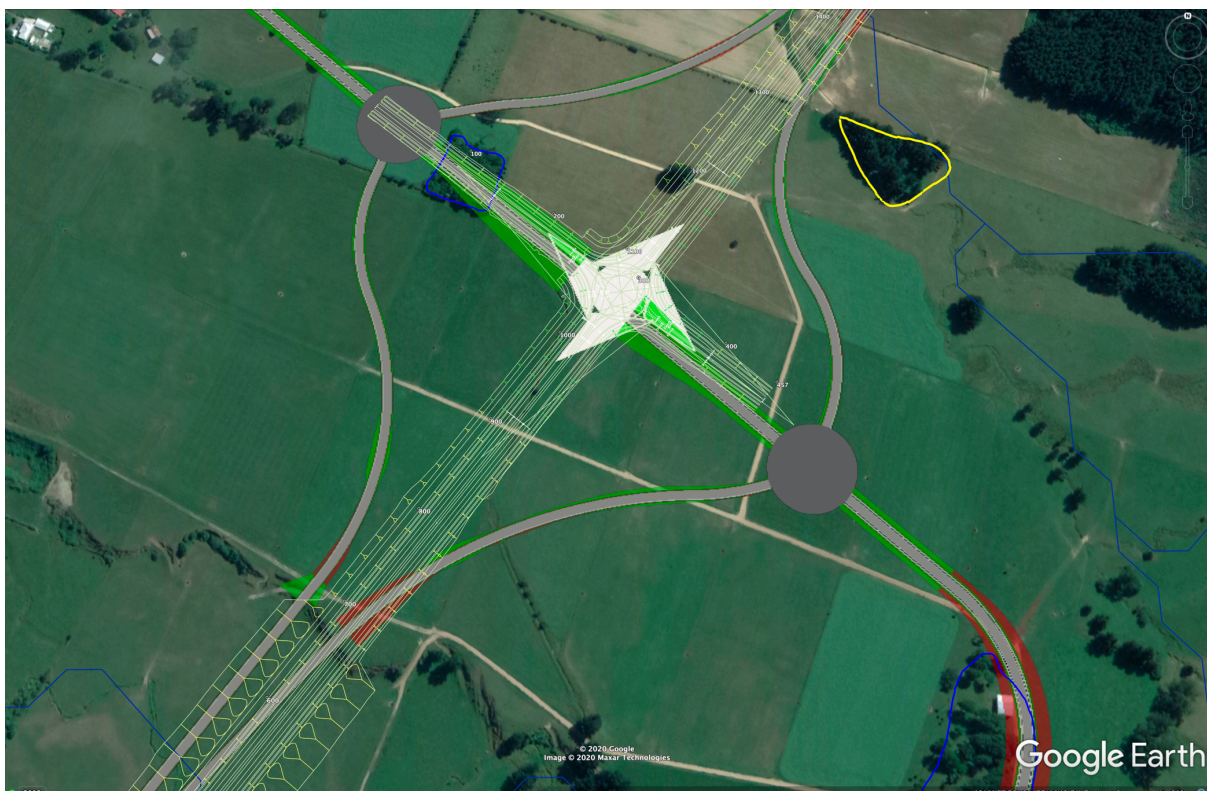
Figure 12. Terrestrial, freshwater and wetland ecological constraints for North Manakau roundabout and grade separation options.
