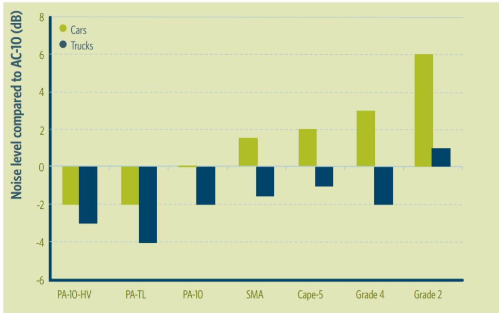
Figure 5 Graph comparing noise reduction attributes of various low-noise surfaces used on New Zealand highways. Reductions are relative to AC-10, this being smooth asphaltic concrete. Grade 2 chipseal included for reference purposes only. Ref; Page 28 NZ Transport Agency Guide to state highway road surface noise .
