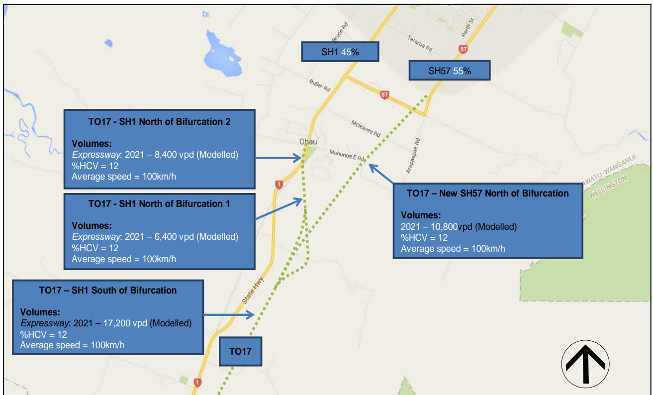
Figure 4: Summary traffic data employed within generic traffic noise predictions [Ref MWH].
