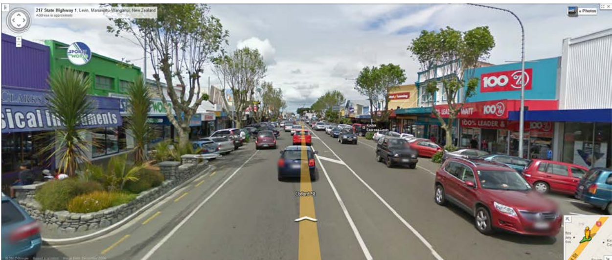
View south along Oxford Street between Queen and Bath Streets (note the parked car reversing out and the waiting car which the red car has passed while using the flush median)
