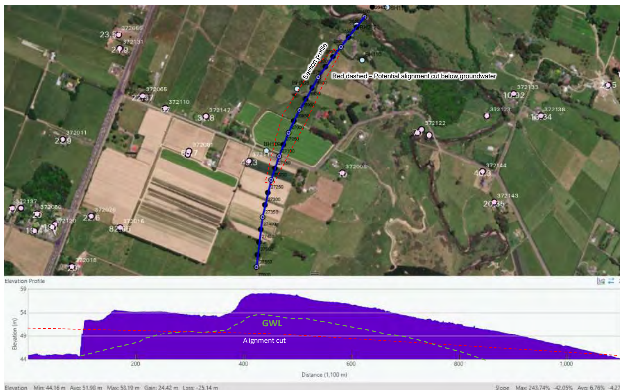
Figure 3-3: Site C - Cross-section and aerial plan showing interpreted GWL, alignment cut, and Horizons bores (shown pink, bore depth centred over point). No wetlands present within aerial image shown
