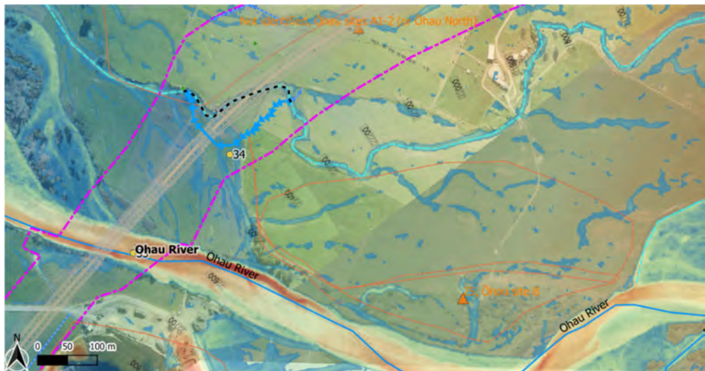
Figure G.38: Existing potential overland flow paths in the wider vicinity of the proposed borrow pit adjacent to the Ohau River.
