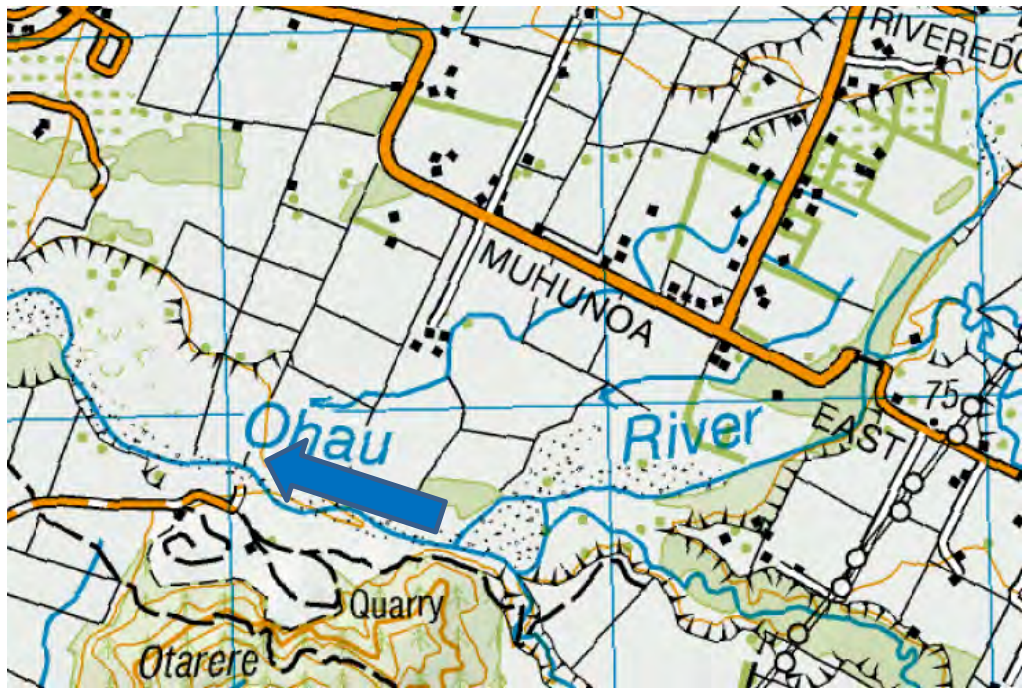
Figure G.39: Location of the potential material supply site just north of the Ohau River, and the inferred groundwater flow direction (blue arrow).
