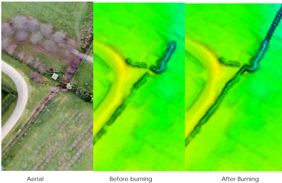
Figure 5-4: Example burning process for a ditch near Waihou Road
