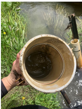
Figure 1: Sample container showing at least 3cm of sediment build up.
