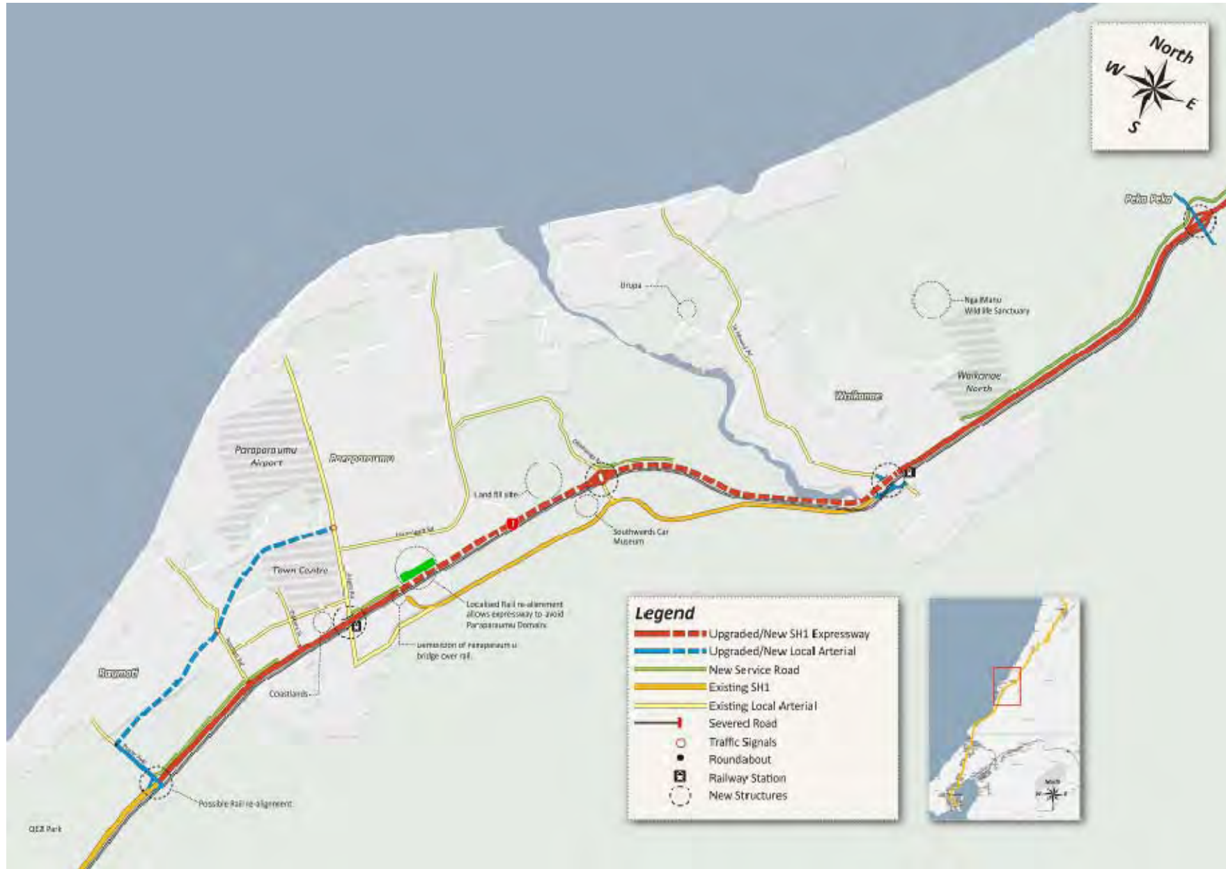
Figure 5.3 – Option 3 - Expressway Follows Rail Corridor
