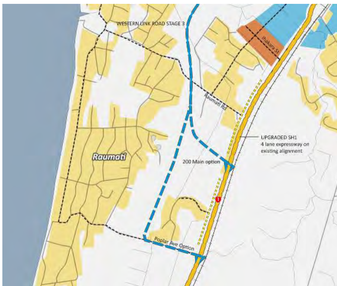
Figure 6.1 – Options for an Interchange South of Paraparaumu
