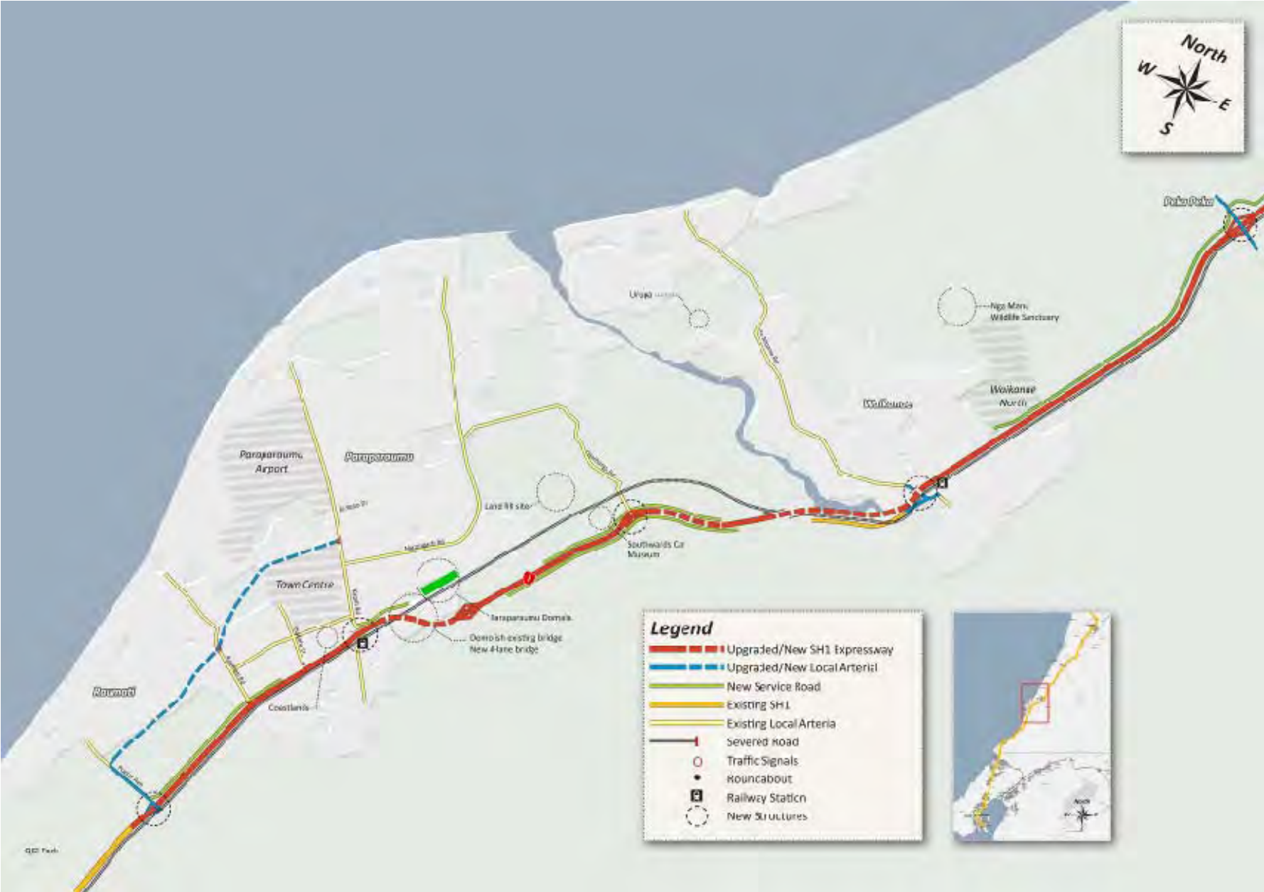
Figure 5.1 – Option 1 - Upgrading the Existing SH1 Alignment
