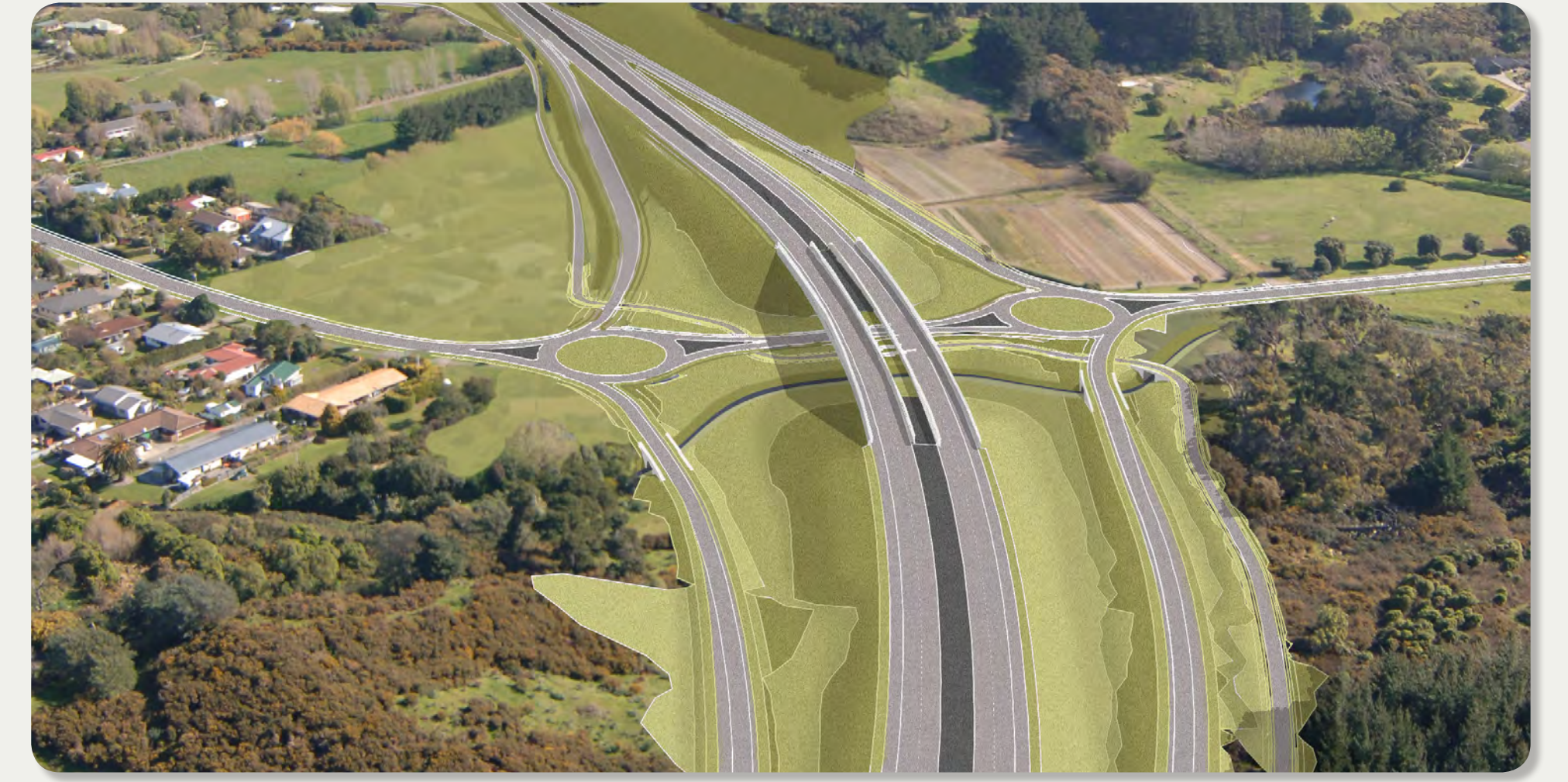
Indicative aerial view of the Te Moana Road expressway interchange. The shared cycle/walk path can be seen crossing from the east to the west (right) side - before mitigation work.
