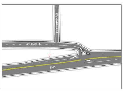
Here's a sketch showing how the temporary access will work. This is indicative only, and is not to scale.
