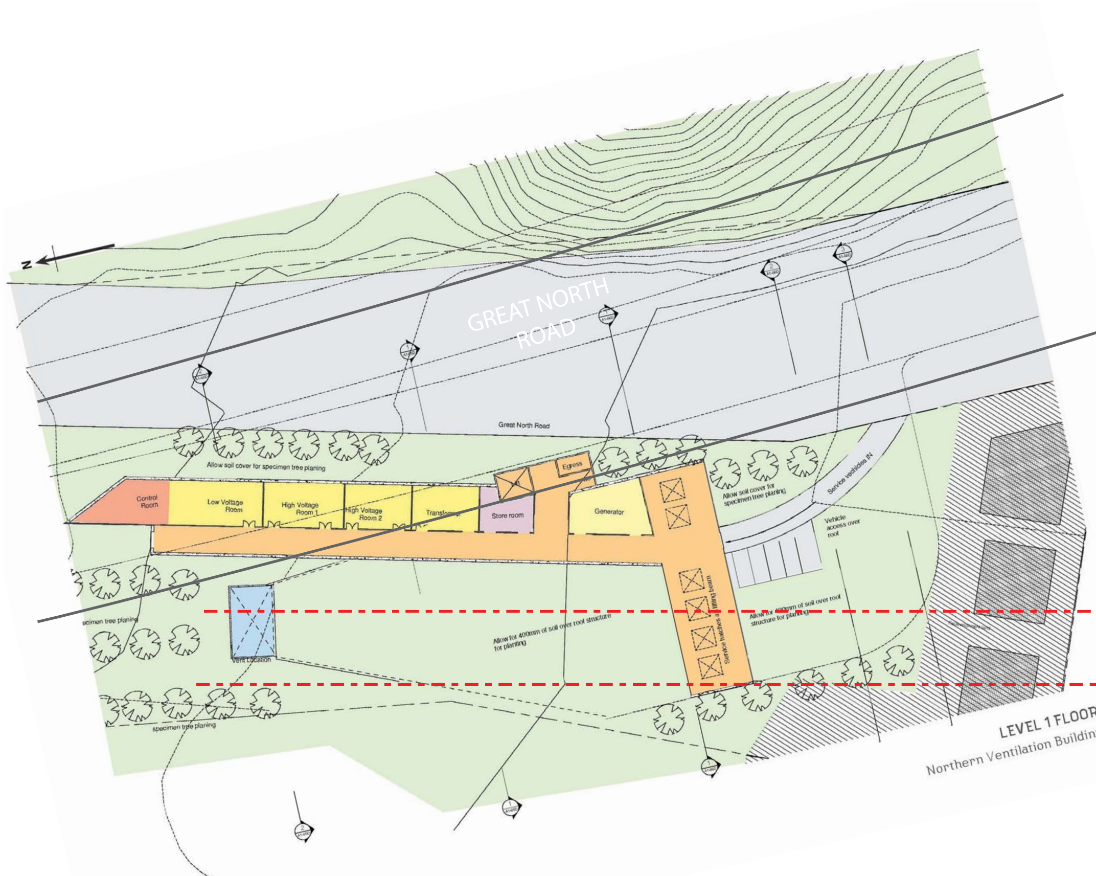
Figure C-7.10: Ventilation building – Great North Road (Concept Option A); ground level plan
