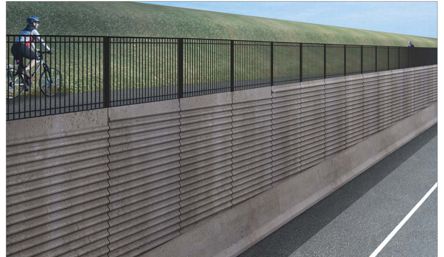
Figure B-21: SH16 retaining wall concept
