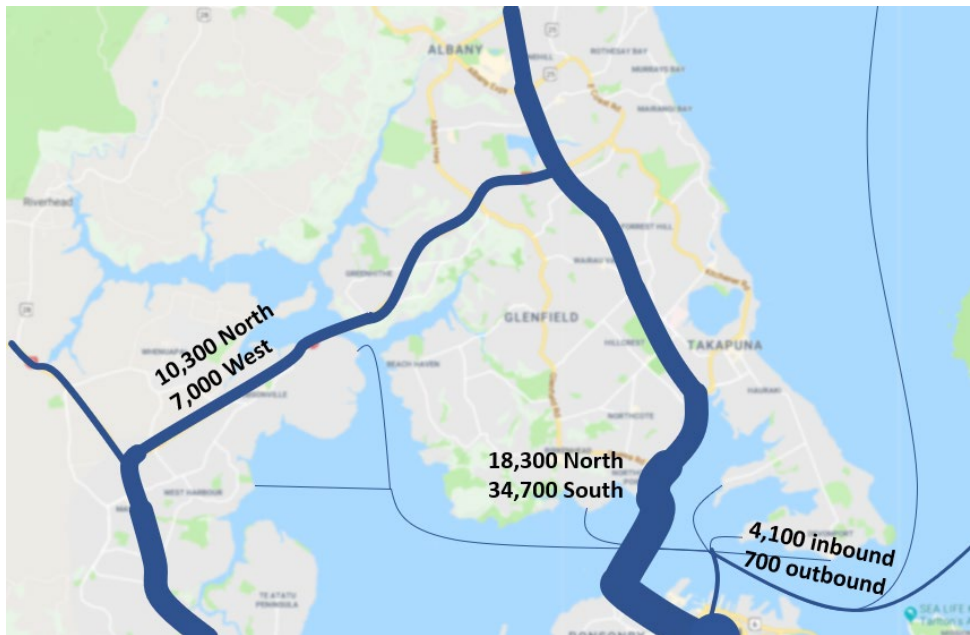
Figure 3 North Shore external travel volumes by corridor, all modes 2048 AM peak (source: AFC)
