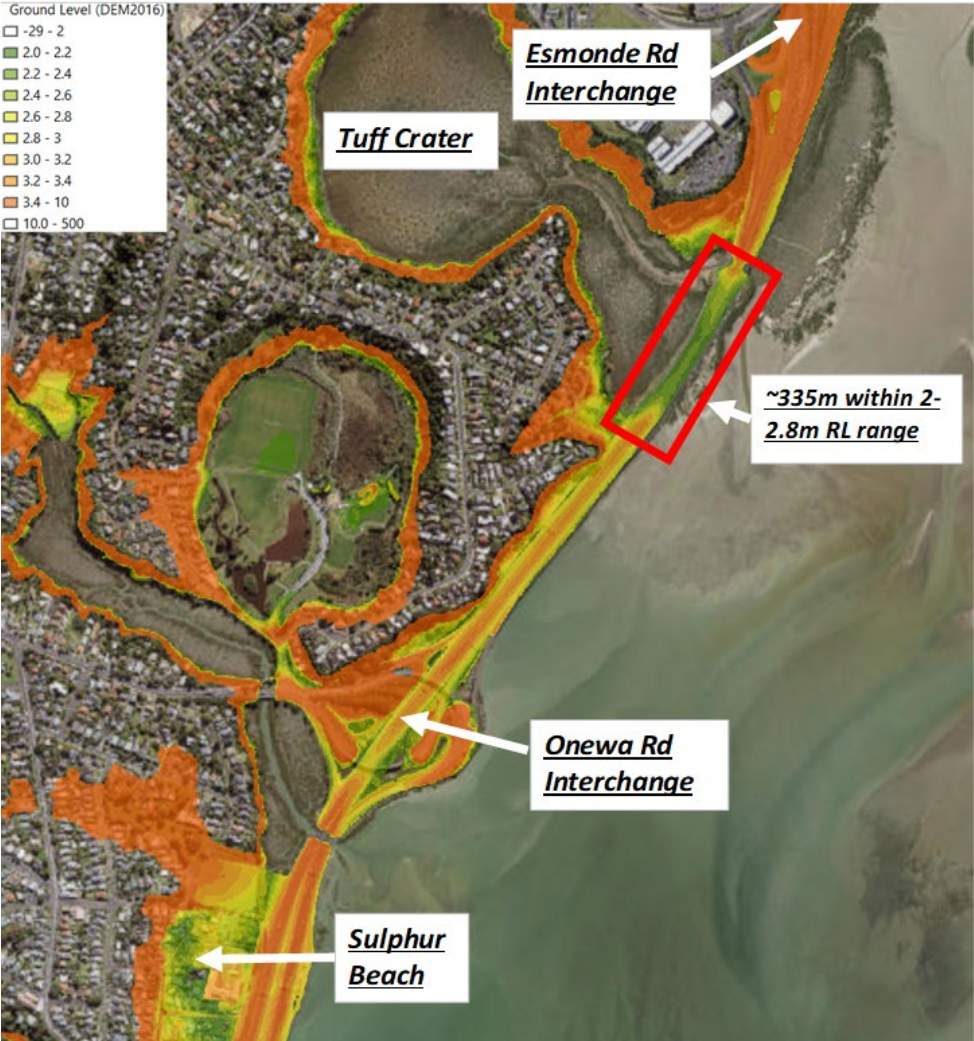
Figure 20: Road Surface Levels (AVD-1946) from DEM 2016
