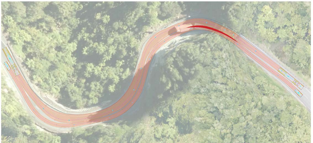
Figure 2.4 – Southbound Semitrailer and Northbound 99% Car through Mt Messenger tunnel
