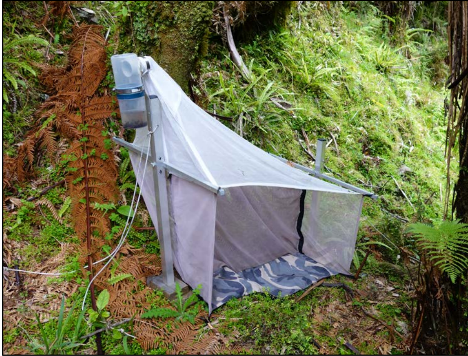
Figure 2.2 – A malaise trap used to collect flying insects, particularly flies, wasps and beetles.
