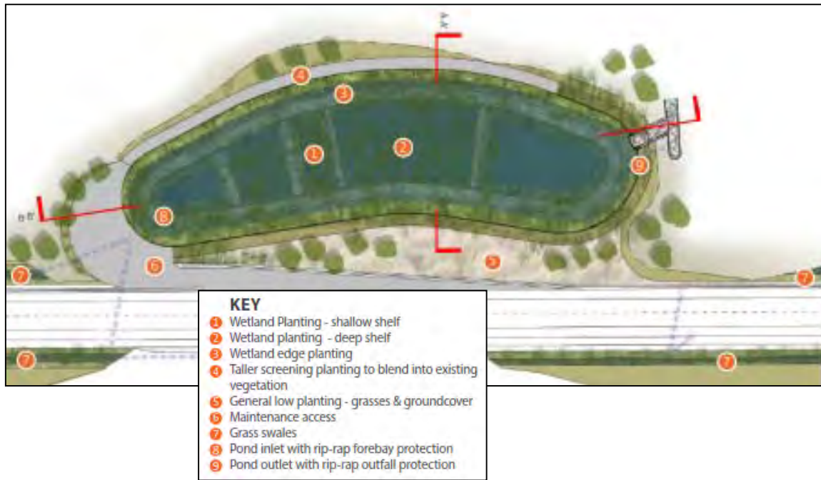
Figure 4.15 – Typical constructed wetland design and planting
