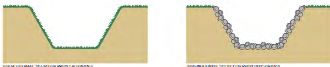
Figure 4.14 – Typical swale design
