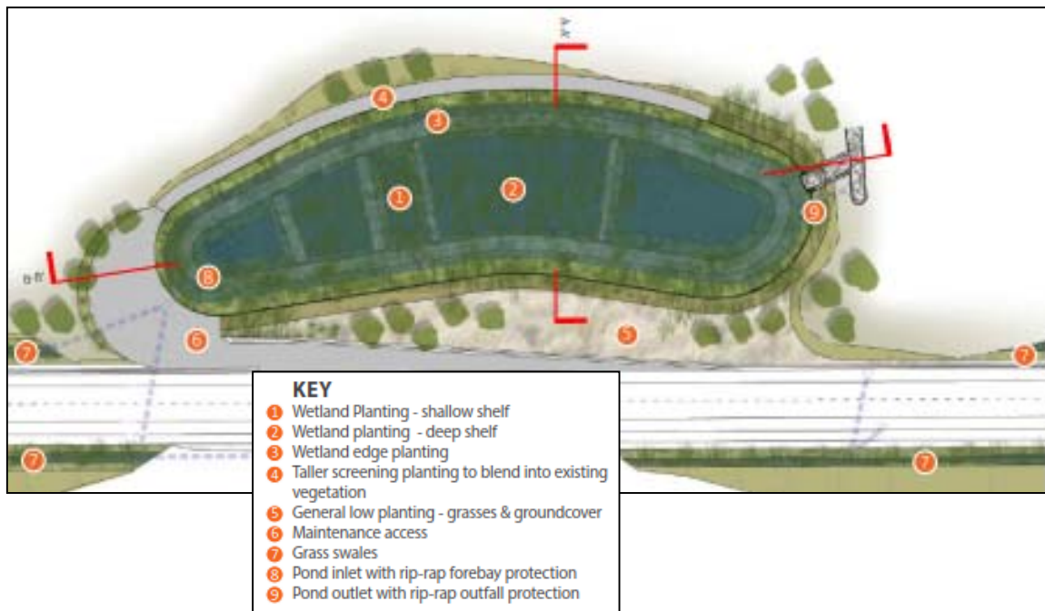
Figure 4.15 – Typical constructed wetland design and planting
