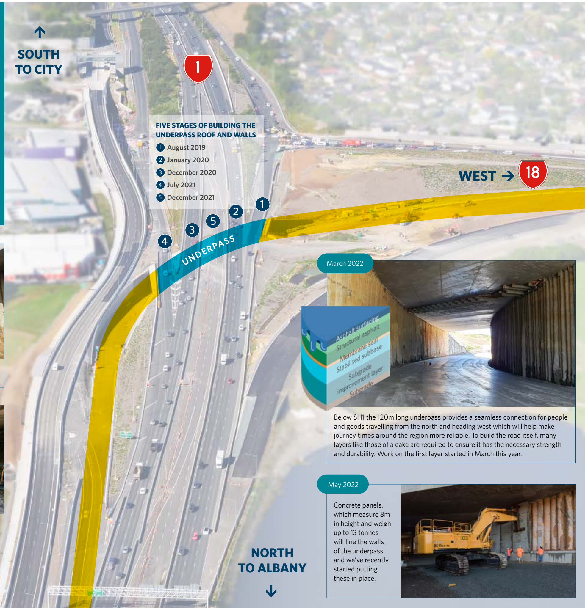
Construction followed a 'top-down' method where the piled walls and roof slab are built first.
