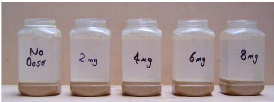
Plate 6 Soil Sample Two Following 30 minutes of Chemical Flocculation (PAC)
