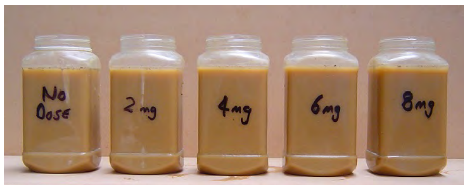
Plate 4 Soil Sample One Following 30 minutes of Chemical Flocculation (PAC)
