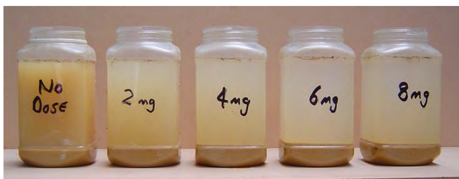
Plate 4 Soil Sample One Following 30 minutes of Chemical Flocculation (PAC)
