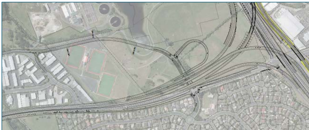
Figure 43 Option 4 - Realignment of PMR with SH18 Eastbound Loop Off-Ramp
