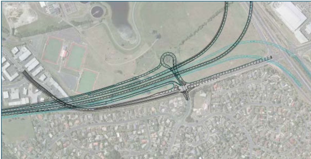
Figure 41 Option 2 – Base Option Variant Incorporating SH18 Eastbound Off-Ramp with Roundabout
