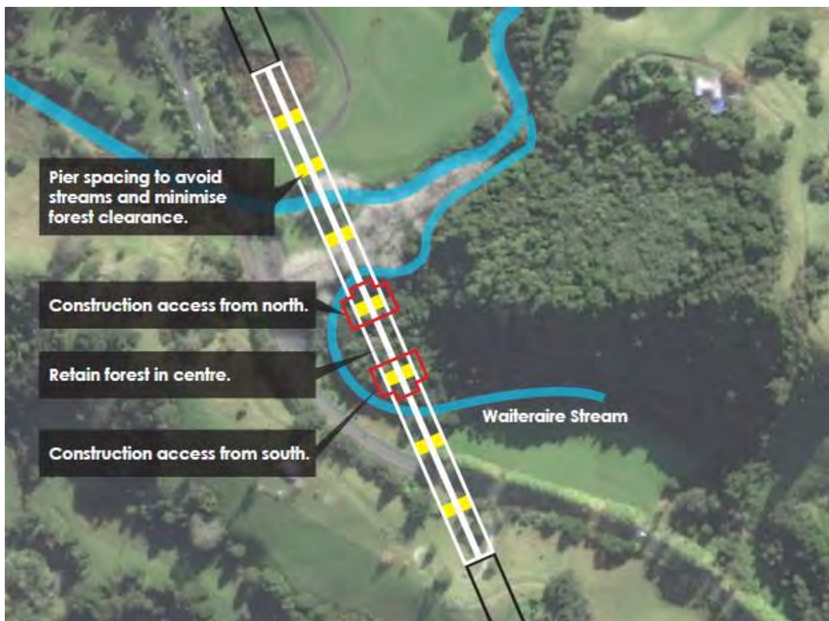
Figure 5-6: Proposed positioning of Bridge 11 piers within SEA
