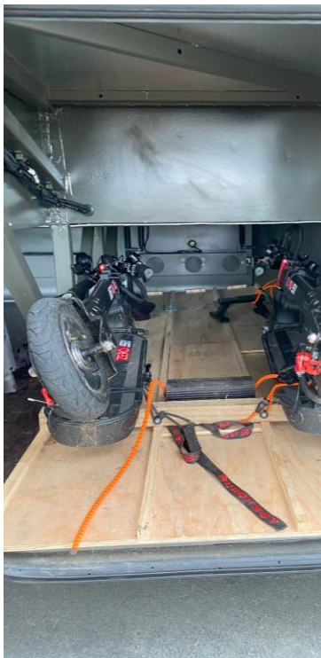
Early prototype of fixed racking system with sliding trays to accommodate six scooters
