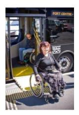
A **wheelchair ramp** is used by someone in a wheelchair to get on and off a bus.
