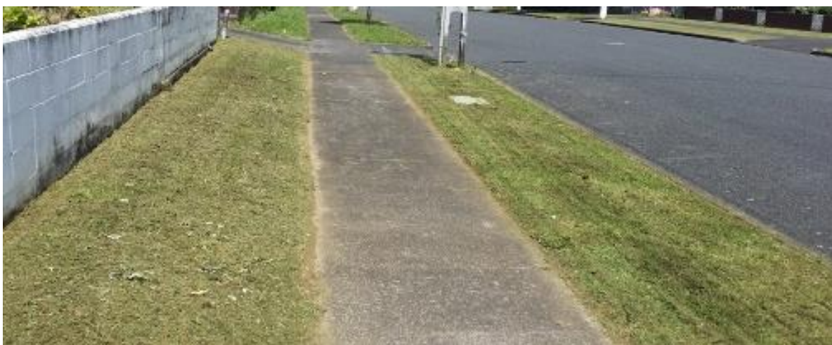
Figure 4A: A berm is a plot of grass, dirt, or garden located beside the roadway.
