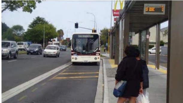
Figure 57: Real-time information display located so passengers can look at it and see the direction of the arriving bus. Source: Auckland Transport.
