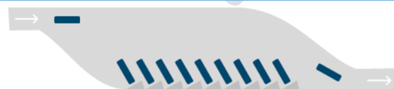
Figure 68: Deep sawtooth or reverse-exit sawtooth (DIRO) at Manukau Bus Station. Source: Auckland Transport.
