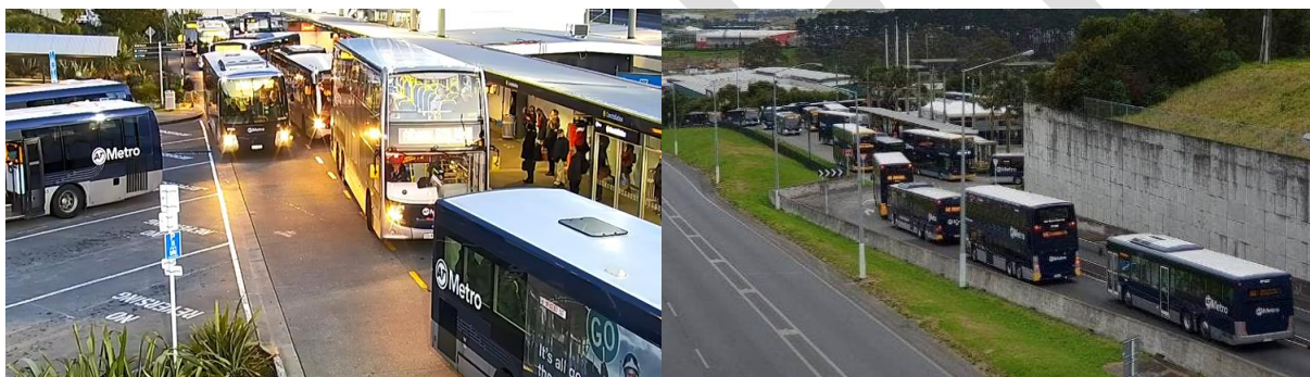
Figure 106: Bus-bunching issues at Constellation Station. Source: Aurecon, Auckland Transport CCTV.
