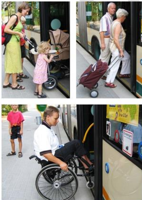
Figure 29: Small gaps between the kerb and bus floor make it easy for passengers to get on or off. Source: Auckland Transport.
