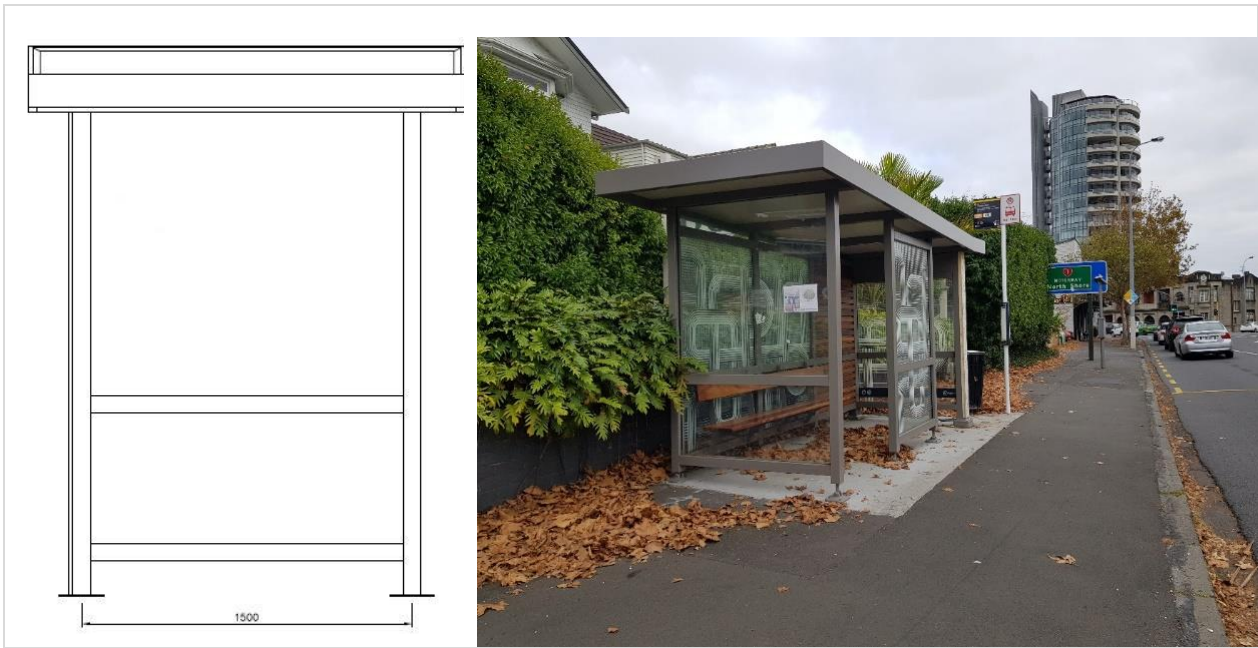
Figure 35: Minor 1500mm shelter. Source: Flow Transportation Specialists.
