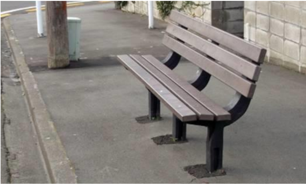
Figure 3: Seat made from recycled plastic materials. Source: Sarah Thorne.
