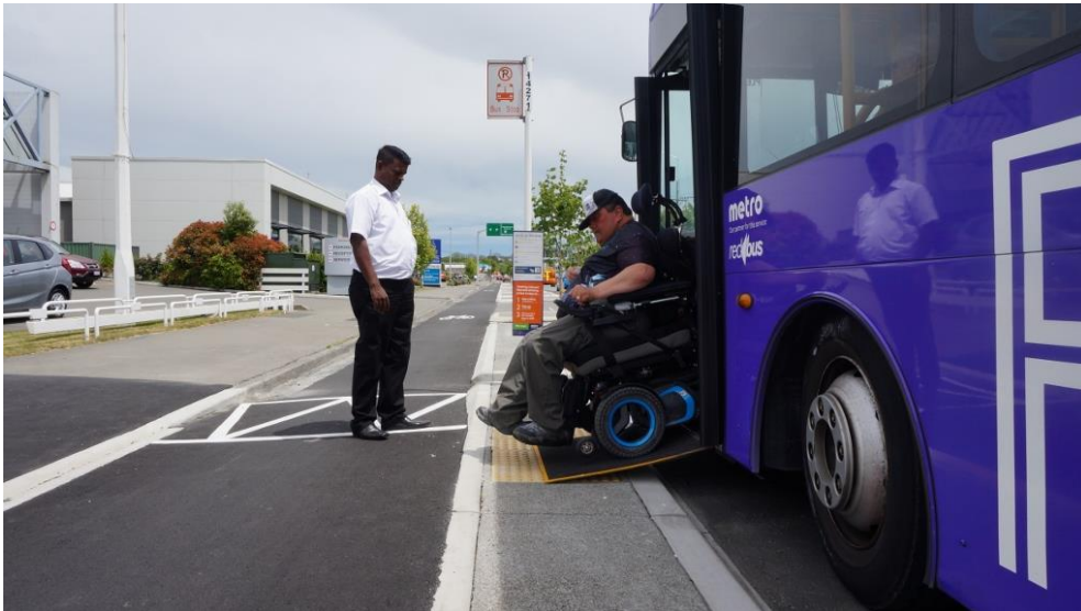
Figure 30: Accessible ramp. Note the narrow width of the boarding island next to the cycleway creates a conflict with the cycleway that the driver is standing on. Source: Brenda O'Donoghue.
