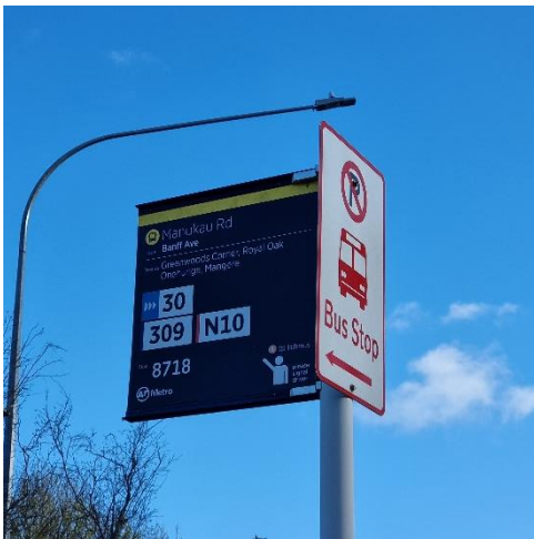
Figure 23: Bus stop sign (R6-71) with supplementary sign. Source: Thomas Chu.
