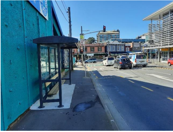
Figure 39: Bus shelter with reduced width of sides to accommodate a clear pedestrian path on a constrained footpath in Wellington. Source: Lorelei Schmitt.
