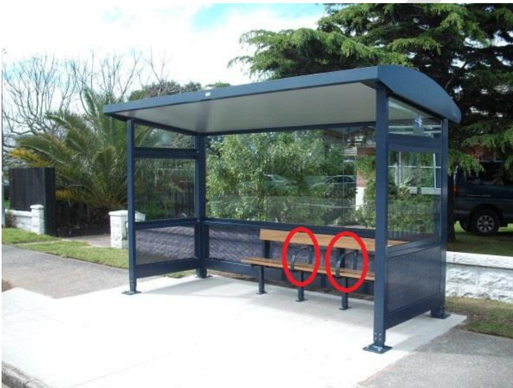
Figure 34: Bus stop shelter with arm rests (circled). Source: ARA Shelters & Structures.
