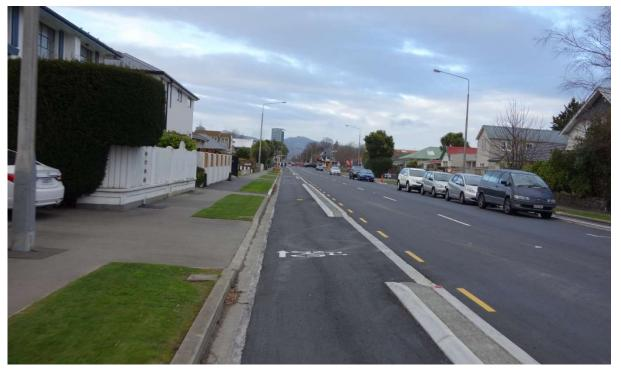
Figure 13: Separated uni-directional cycleway without adjacent parking at a residential driveway
