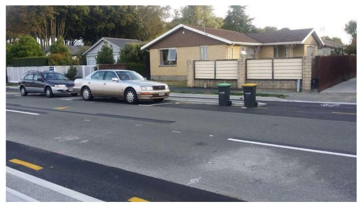
Figure 17: Applying setbacks for parking at driveways along separated cycleways, Strickland St, Christchurch
