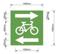
Figure 19: Symbol for two-way cycleway at narrow driveway for a two-way cycleway (i.e. <3.1m wide)
