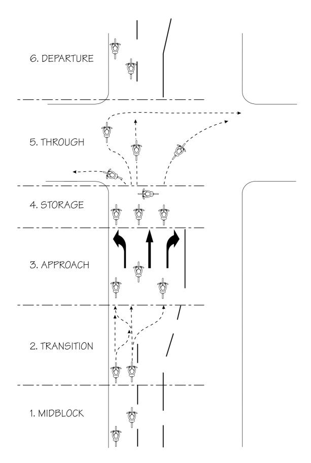
Figure 1. The model bicycle intersection and its six elements
