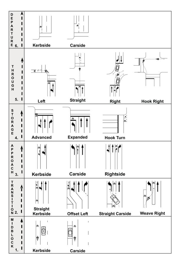
Figure 2. Options within the six elements of the "model bicycle intersection"
