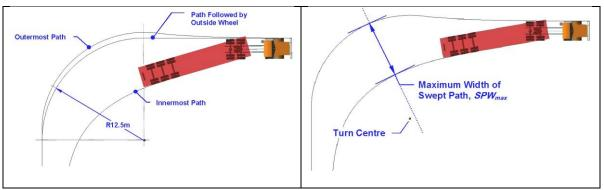
Figure 1. Illustration of the swept width performance measure reproduced from (National Transport Commission 2007)
