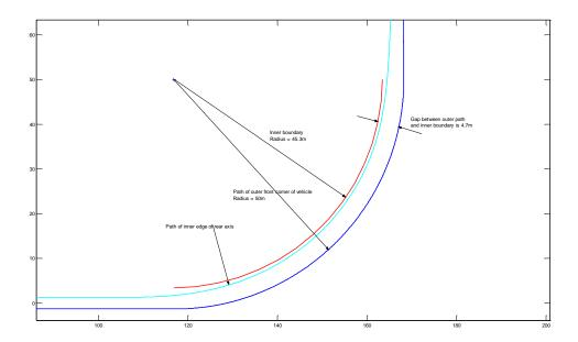
Figure 4. Swept path requirements for a maximum category 1 overdimension vehicle
