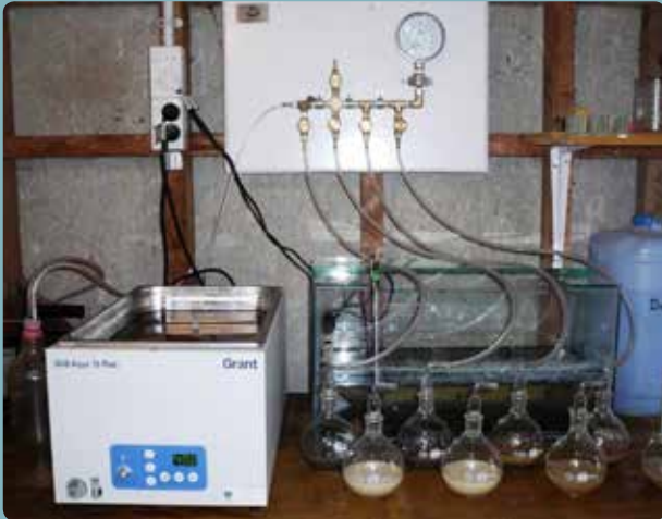
One of the many tests performed in the lab - this vacuum test determines the solid density of soil particles
