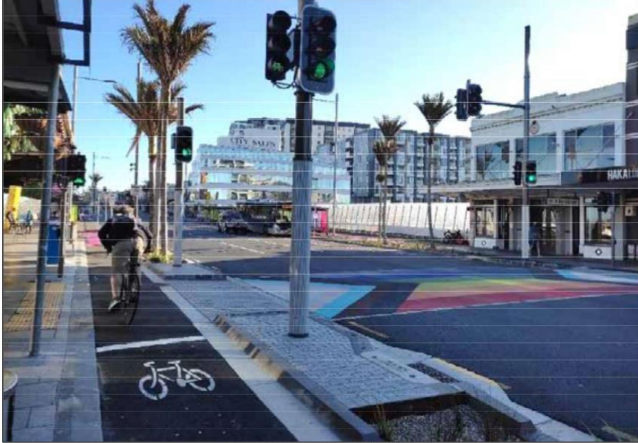
Figure 4 Separated cycle facilities
